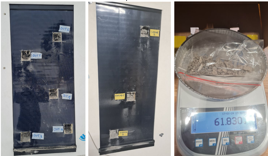
Figure 24. Destructive opening of the outdoor facade after 20 months of measurements (left) and similar opening conducted in the climate chamber (middle). PCM mortar pieces removed from each sample slot were sealed in plastic bag until first weighting (right).
