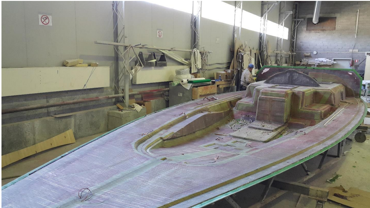
Figure 3.5 The laminated deck upside down.
