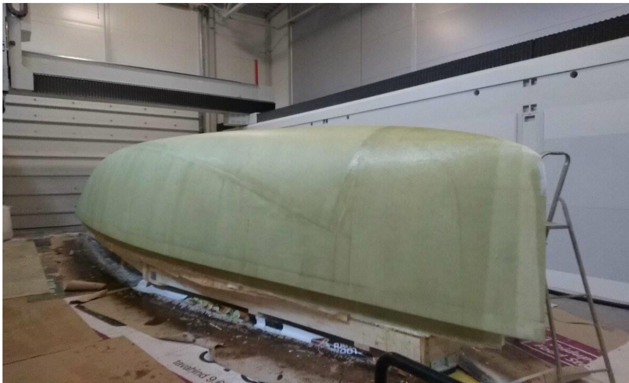
Figure 3.4 CNC machined plug, covered with GRP
