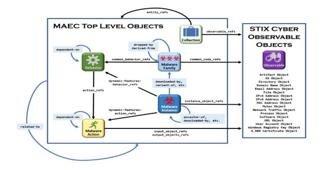
Figure 10. MAEC Top Level Objects and relationships with STIX observables. Source: [61].
