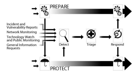
Figure 2. High-level incident management processes. Source: [12].
