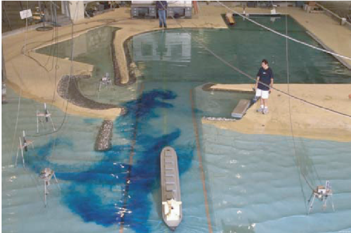
Figure 4. Three dimensional physical modelling, two ship models are used [Coastal Engineering Manual, 2002].
