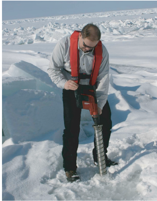
Figure 3. Obtaining a drilling core for ice thickness measurements.
