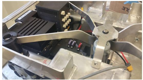
Fig. 2. The lifting mechanism.
