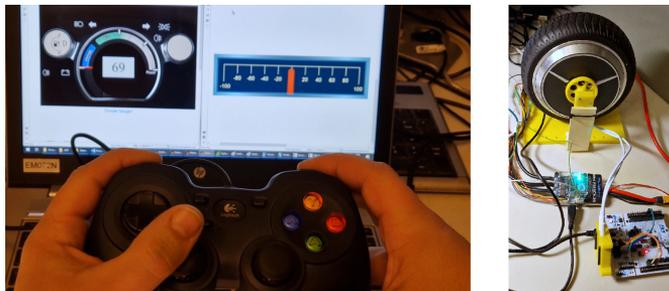
Figure 27: HIL test setup.
