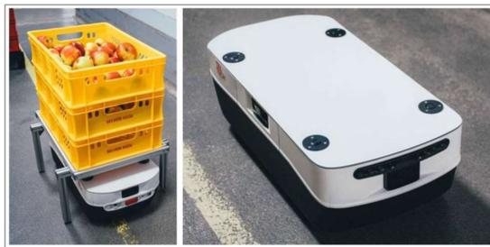
Fig. 1. Universal easily expandable logistics robot prototype "BoxBot".
