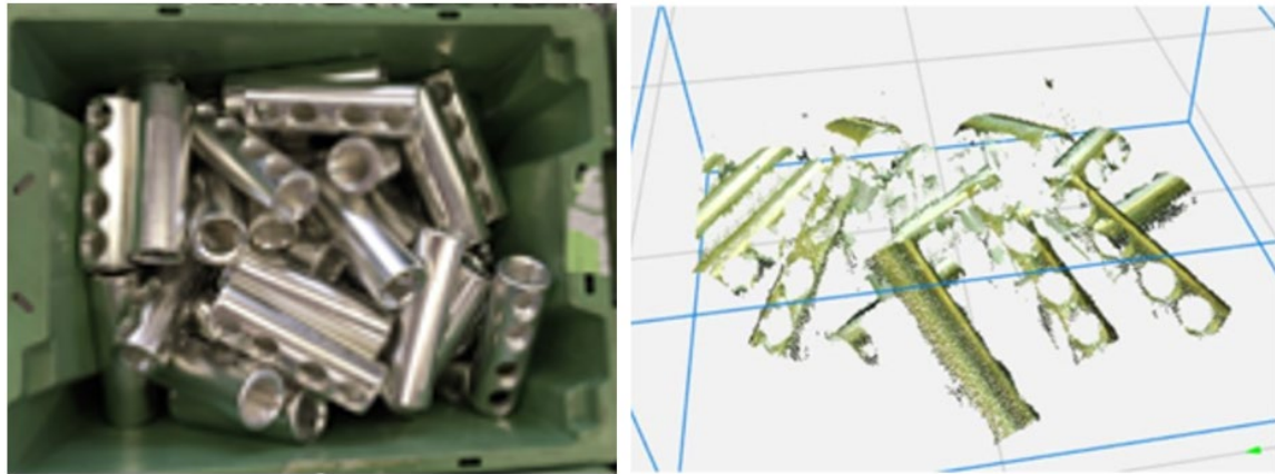
Figure 4.16 A lot of reflection from cylinders lying in the bin. Some cylinders have a lot of distortion.
