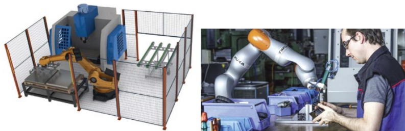
Figure 2.5 industrial robot on the left - safety fences are required to prevent harming humans. Collaborative robot on the right - allow human worker to work together [17]
