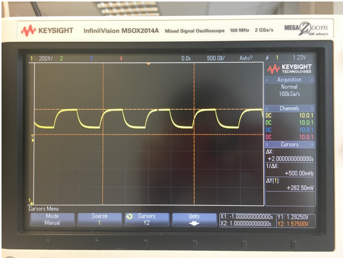
Figure 33. The output voltage of Photodiode circuit
