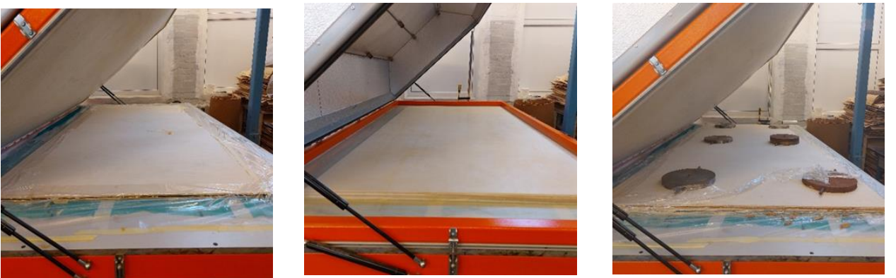
Figure 3. left: the top plywood is glued and ready for pressing. middle: panel under the press. right: pressed panel.
