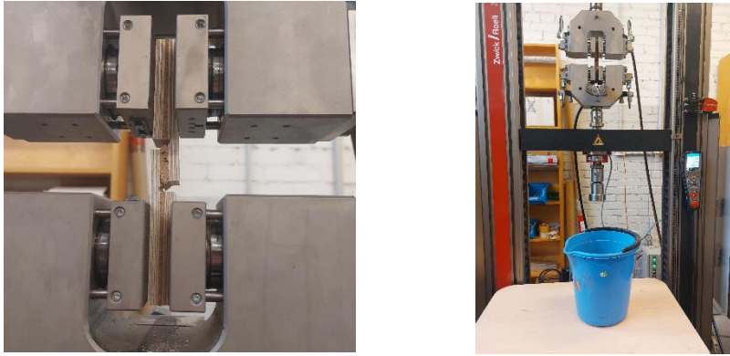
Figure 19. left: the dry sample with cork core material is tested. right: the wet sample with Amorim cork core material is tested.
