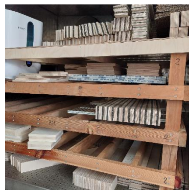
Figure 5. Left: samples are cut. Right: samples are conditioned in the climate chamber.
