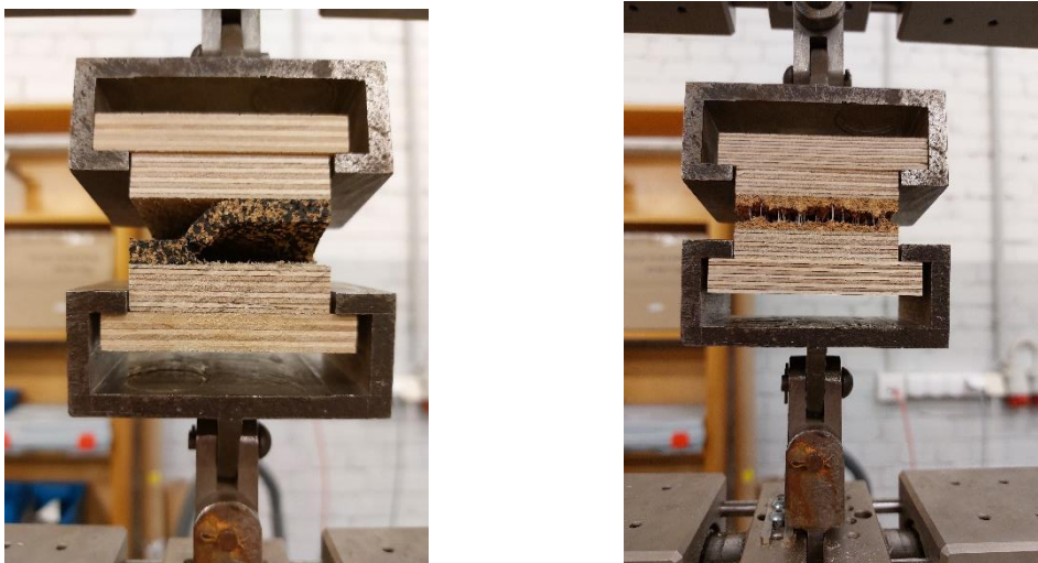
Figure 16. Left: Mixed failure. right: core failure.
