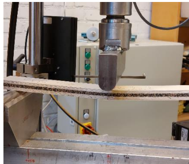
Figure 8. The sample with rubber cork 6 mm thicknesses is tested according to EN 314.
