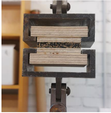
Figure 7. The sample with rubber cork 6 mm thicknesses is tested according to EN 319.
