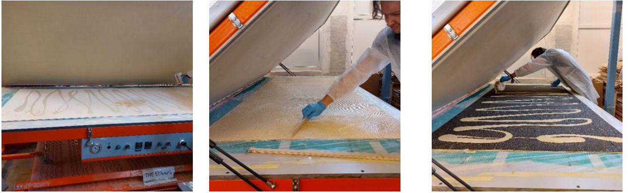
Figure 4. Left: Application of glue on the surface of the plywood. Middle - Spreading of glue on the side of the plywood. Right - Application of glue on the surface of the core material.
