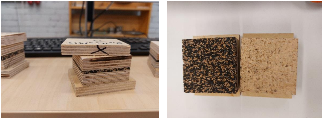
Figure 15. Left: plywood holder failure. right: adhesive failure.
