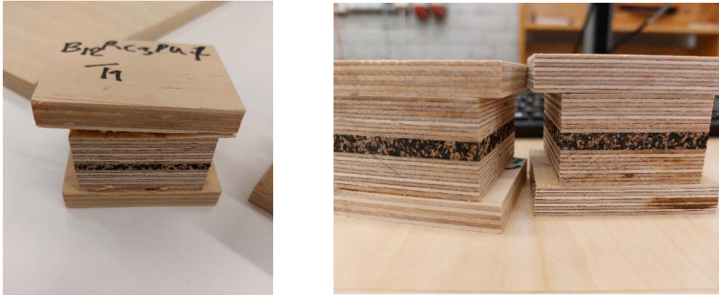
Figure 17. Left: plywood failure right: core failure.
