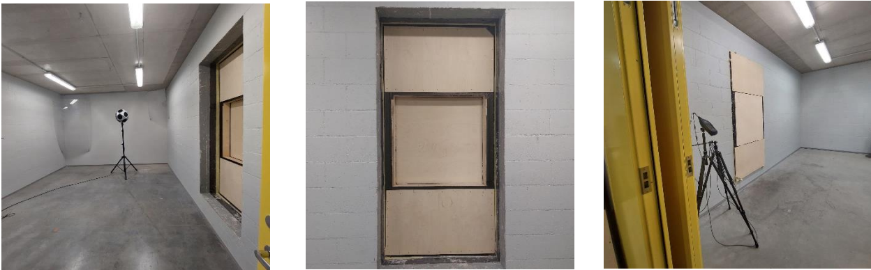
Figure 6. Left: noise source room, sound source. Middle: opening is of laboratory (test sample presented is not belonging to this test). Right: receiver room with microphone.
