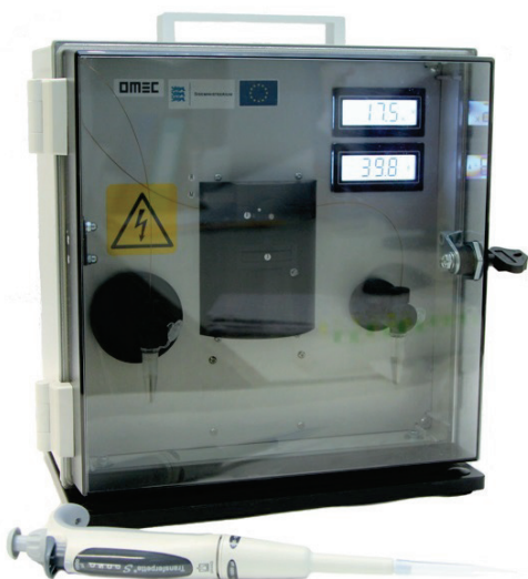
Figure 3.3. The new portable UVC excitation fluorescence CE instrument.
