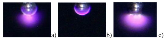
Fig. 12. Corona images of a 14.5 mm sphere 8 cm above the ground plane. a) AC supply at 31.8 kV peak. b) +DC supply at 30 kV. c) -DC supply at -30 kV.
