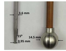
Fig. 2. Detail of the needle and sphere electrodes analyzed in this work.
