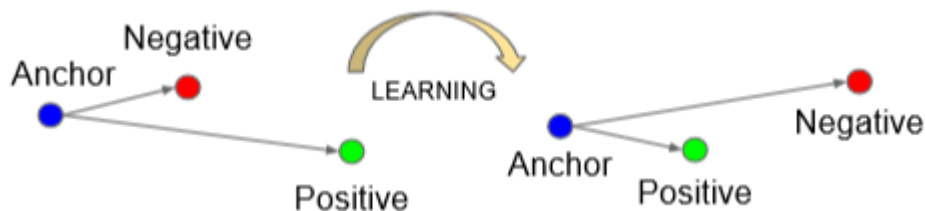
Figure 5.1 Before and after applying triplet loss
