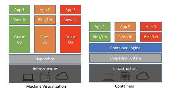
Figure 12 Difference between virtual machines and containers[2]
