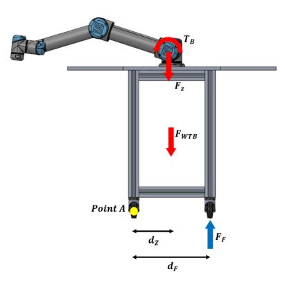
Figure 3.5 Internal forces of test bench for first draft
