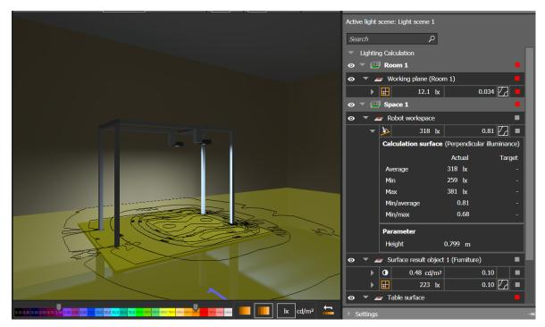
Figure 17.8 Results obtained for the first simulation
