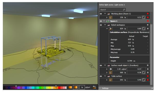
Figure 4.12 Results obtained when the light of the room is added
