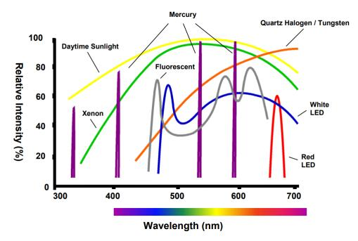
Figure 2.9 Wavelength vs Relative Intensity of light sources [16]
