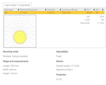
Figure 4.11 DSP52-18-041 Optima EM3 940 specifications from the ASTZ manufacturer [55]
