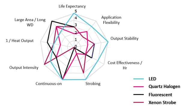
Figure 2.8 Comparative graph of illumination sources [16]
