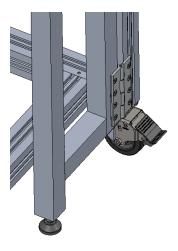
Figure 3.7 Retracted leg position
