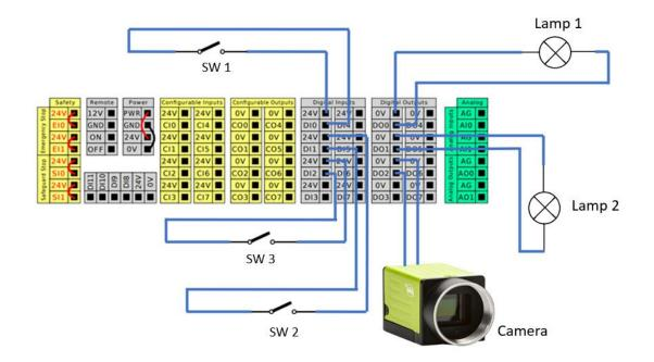
Figure 5.1 Electrical circuit for two HSI LED
