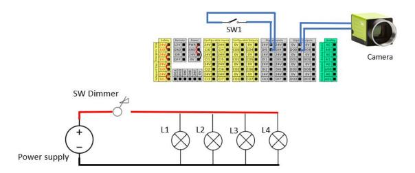
Figure 5.3 Electrical circuit for four halogen lamps
