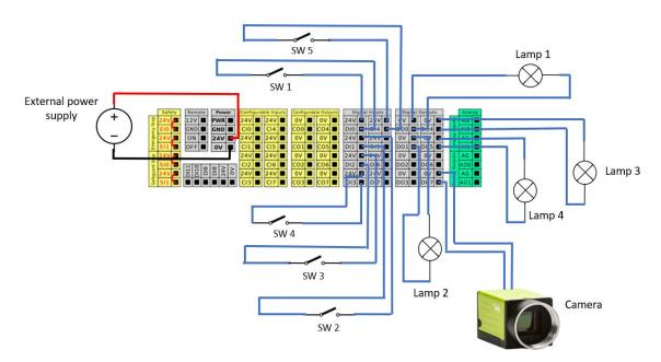
Figure 5.2 Electrical circuit for four HSI LED
