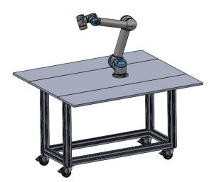
Figure 3.3 Preliminary design of the test bench
