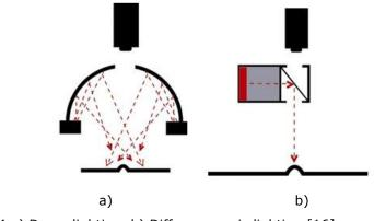
Figure 2.14 a) Dome lighting, b) Diffuse on-axis lighting [16]
