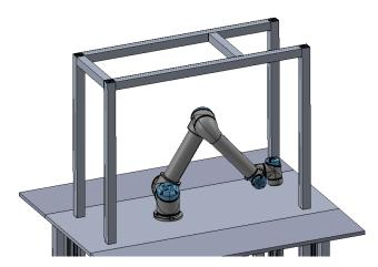
Figure 3.10 Arches to place lights and cameras
