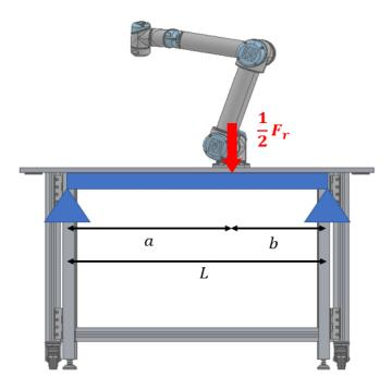
Figure 3.9 Scheme of forces to calculate deflation a and b – length from the point load to one end of the beam, E – modulus of elasticity of the material, I – moment of inertia based on the shape of the extrusion, L – total length of the beam.
