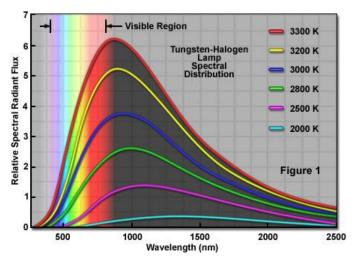
Figure 4.1 Spectral distributions of halogen lights [47]
