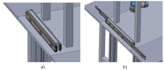
Figure 3.11 Sliding system, a) slider closed and b) slider opened
