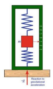
Figure 4 Gravitational force measurement of an accelerometer [10].
