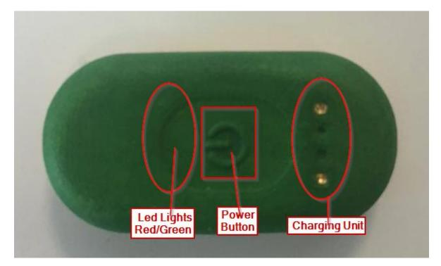
Figure 13 BLE Wearable Sensor.
