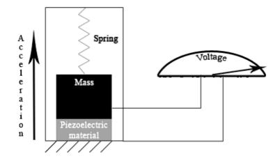
Figure 6 - Applied acceleration trigs voltage generation for piezoelectric material [8].
