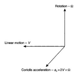
Figure 8 Coriolis acceleration which is generated by linear motion and rotation[15].
