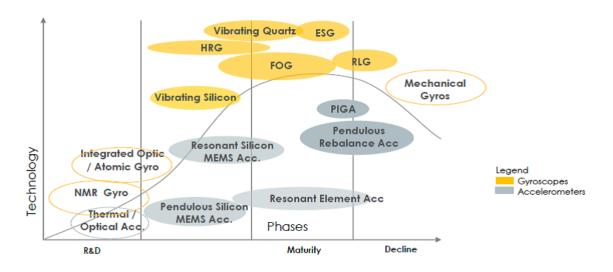
Figure 7 Development of accelerometer and gyroscope technology [15].
