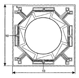
Figure 10 Structure of resonant ring gyroscope [15].
