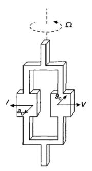
Figure 9 A structure of a simple tuning fork [15].
