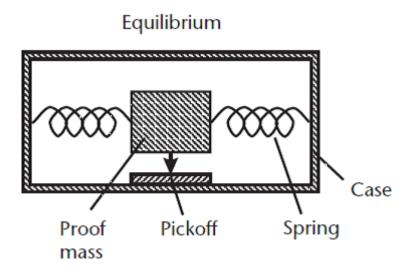
Figure 2 Components of an accelerometer at equilibrium state [7].
