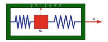
Figure 3 Linear acceleration is applied to an accelerometer [10].
