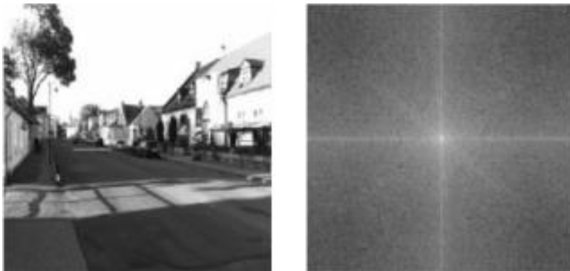
Figure 2.7. An image of a city landscape and visualization of its amplitude spectrum
