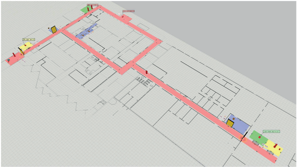
Figure 2. AMR pathways setup on factory layout (setup a: for red boxes)
