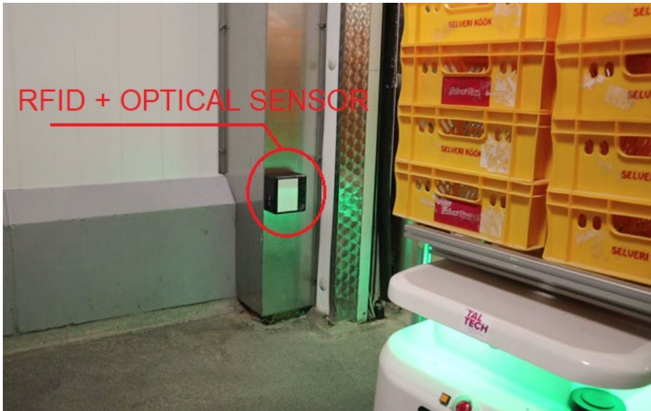
Figure 17. Implementation of RFID and optical sensors in the chemical industry case, enabling automatic identification and synchronization of transport tasks with AMRs (adapted from Publication I).
