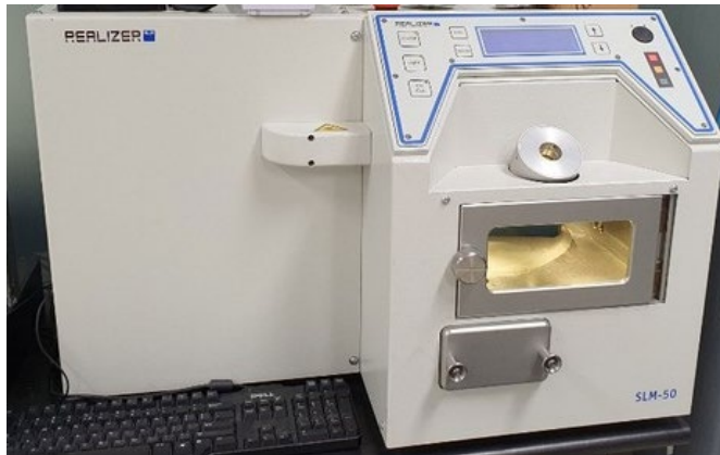
Figure 2.1 ReaLizer SLM 50 device used for the fabrication process.
