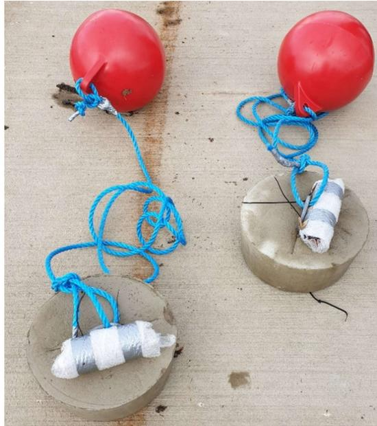
*Figure 3.2. Pressure gauges*
