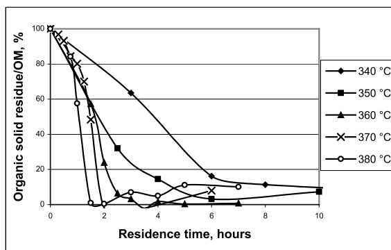
Fig. 1. Effect of time on the distribution of initial OM between TB (a), gas (b) and organic solid residue (c) at different nominal temperatures, °C.
