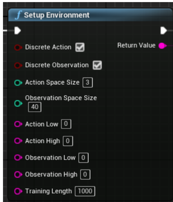
Figure 4.9 Blueprint node for compiling environment message
