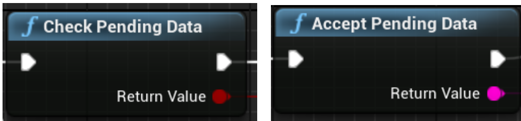
Figure 4.5 Blueprint node for listening and accepting a data
