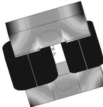
Figure 3.17 A 3D model of a high-frequency transformer solved by *MagNet* software (*Infolytica Ltd*)
