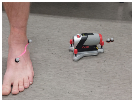
(b) Utilizing a laser for enhanced precision in marker placement for gait analysis
