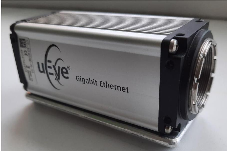
Figure 3. 1 uEye Camera used in this thesis
