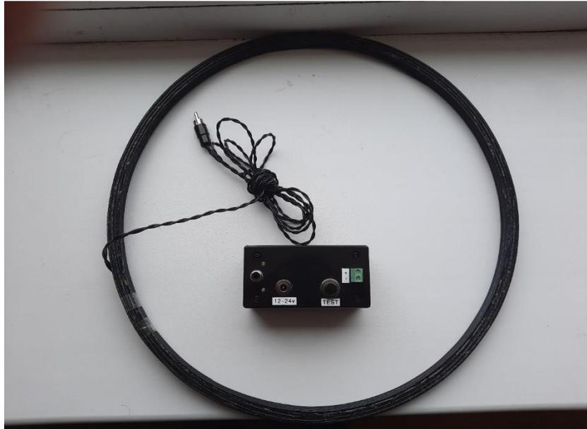
Figure 3. 4 Electromagnetic pulse coil
