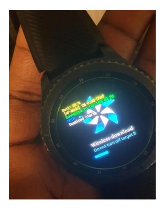
Figure 6 Device connected to computer and downloading a custom ROM
