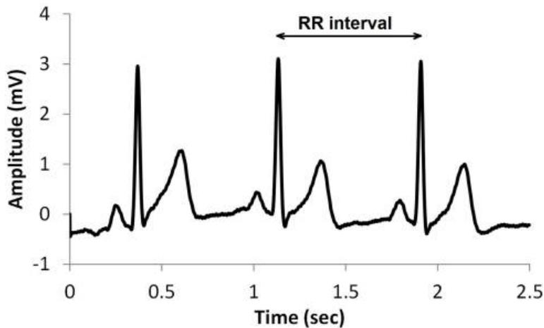
Figure 2. The ECG-signal and RR-interval
