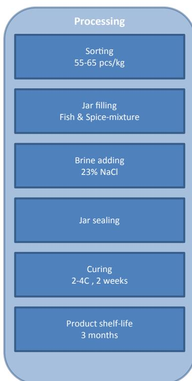
**Figure 1** – Production scheme of spice-cured sprats “Sprats of Tallinn”.
