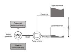
Figure 3. Schematic diagram of pumped hydro storage system
