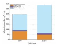
Figure 14. The annualized life-cycle costs for long-term ESSs. The systems are rated at 100 MW/600 MWh, and are deeply discharged once per day throughout the project horizon. [13]
