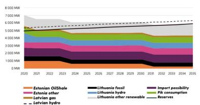
Figure 18. Baseline scenario for the Baltic synchronous area [1]
