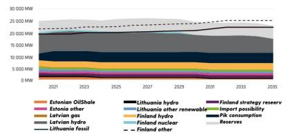
*Figure 17. Available production and transmission capacities in the Baltics and Finland in the period 2020-2035* [1]
