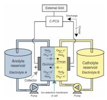
Figure 11. The operating principle of flow batteries. [13]
