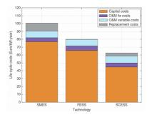
Figure 16. The annualized life-cycle costs for short-term storage systems. The systems are rated at 1 MW/0.003 MWh, taking 50 000 equivalent discharge cycles per year into consideration. [13]
