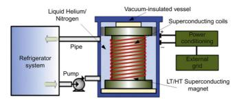
Figure 7. Schematic of distributes SMES system [16]
