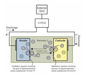
Figure 10. The operating principle of battery
