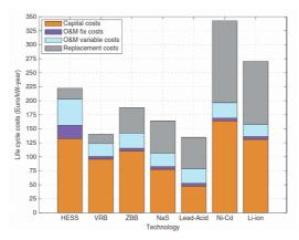
Figure 15. The annualized life-cycle costs for long-term storage systems. The systems are rated at 10 MW/10 MWh, and are deeply discharged once per day throughout the project horizon. [13]
