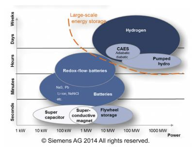
Figure 2. Overview of storage technologies and their typical power and capacity ranges.
