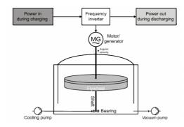
Figure 5. Schematic diagram of flywheel energy storage system
