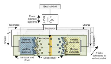
Figure 6. The illustrative topology of a supercapacitor, depicting the electrical double layers at each electrode/electrolyte interface [13]
