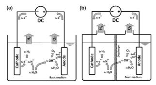
Figure 8. (a) Basic principle of an open EL cell in basic medium. Stoichiometric factors are related to the generation of one molecule of oxygen. As the half-cells are open oxyhydrogen is produced. (b) Deploying a semipermeable diaphragm between the two half-cells allows the separation of the two gases. [11]
