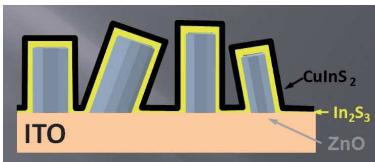
Figure 1. A sketch of the structure of the \text{ZnO}_{\text{NR}}/\text{In}_2\text{S}_3/\text{CuInS}_2 solar cell deposited by spray sprayed onto ITO. The \text{CuInS}_2 absorber is covered with graphite paste (not shown). The SEM images of partially completed \text{ZnO}_{\text{NR}}/\text{In}_2\text{S}_3 cell (Figure 17) and of the completed cell (Figure 21) follow later near the relevant discussion. Further SEM images and an EBIC (electron beam induced current) image of the structure can be found in [130] and in [V] (Appendix A).
