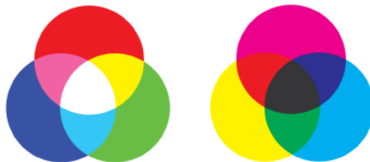
Figure 2.1.5 - RGB additive color model (left) and the CMYK subtractive color model (right)
