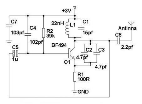
Figure 5. Mobile phone jammer<sup>1</sup>
