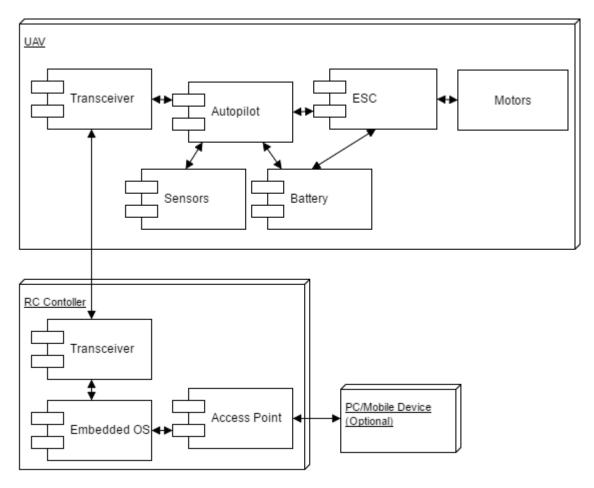
Figure 4. Mini UAS system architecture
