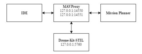
Figure 9. Lab setup
