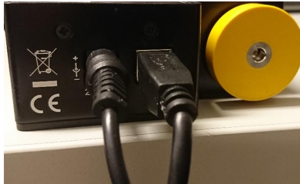
Figure 14 – LTS300/M wiring. Power supply(left), USB(right).
