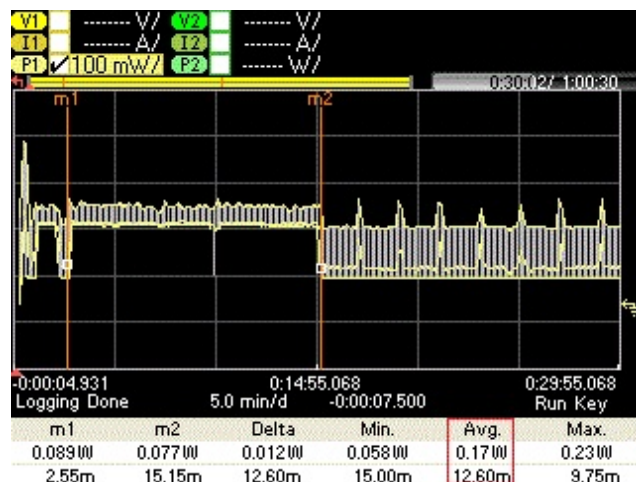
Figure 1. Power graph of the BG96 NB-IoT module when transmitting an image ( 1600 \times 1200 pixels, 357.17 kB). A total of 239 transmissions are needed (12.60 m) with an average power of 0.17 W, which translates to an energy consumption of 0.0357 Wh.
