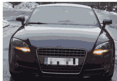
(b) Output image from the K_Means algorithm for K (colors) = 10: Size: 31.6 kB approx.
