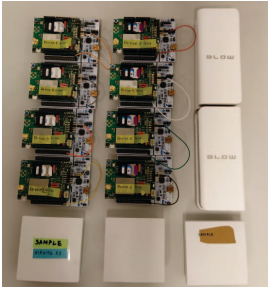
Figure 3: Some of the NB-IoT (uncased) and Sigfox nodes, and batteries
