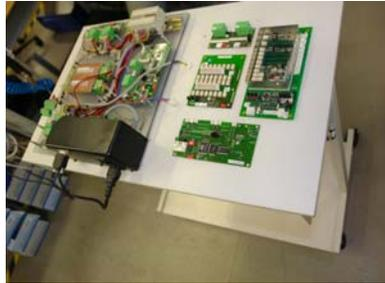
Figure 2.9 Pre-testing station for PWB modules
