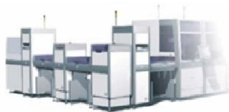
Figure 4.3 With standard module frames composed assembly line
