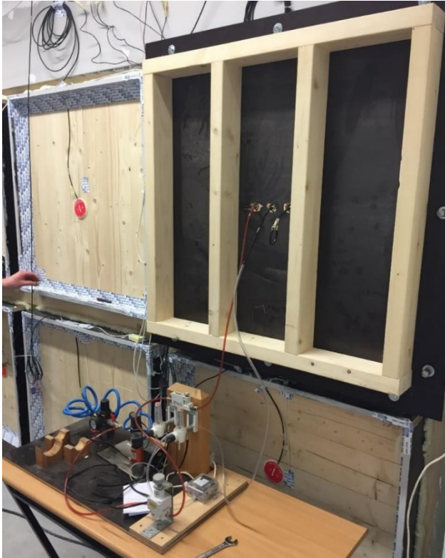
Figure 2.10: A scheme of the apparatus to be used for the air permeability test
