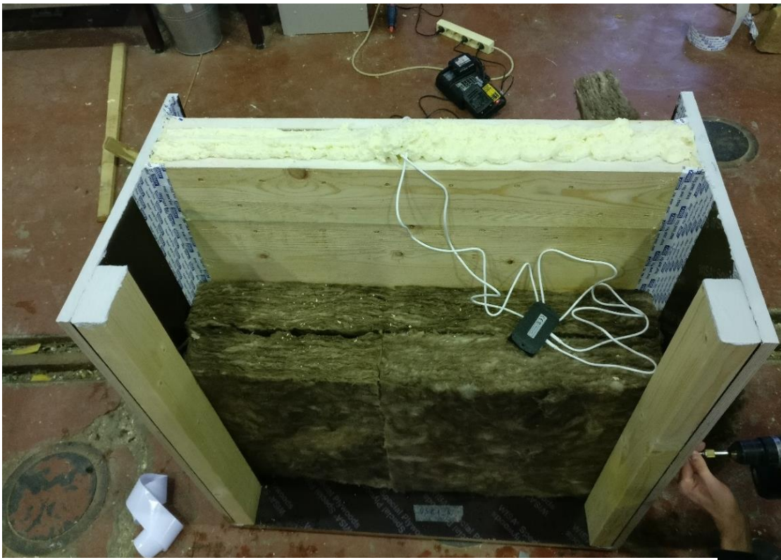
Figure 2.6: One of the test wall used in the research with mineral wool as insulation
