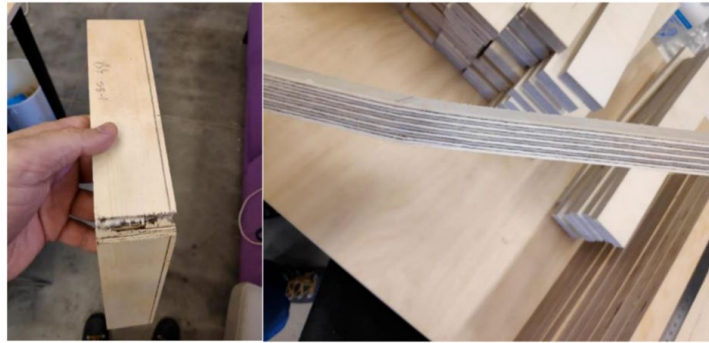
Figure 9. Test pieces after bending tests, showing brittle failure in black alder (left), and ductile failure in aspen (right) plywood.
