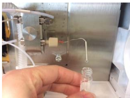
Picture 1. Isolation of oligomers by collecting the fractions from the HPLC apparatus.
