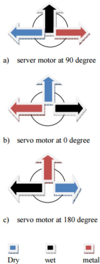
Figure 10. Rotation of circular base of servo [7]
