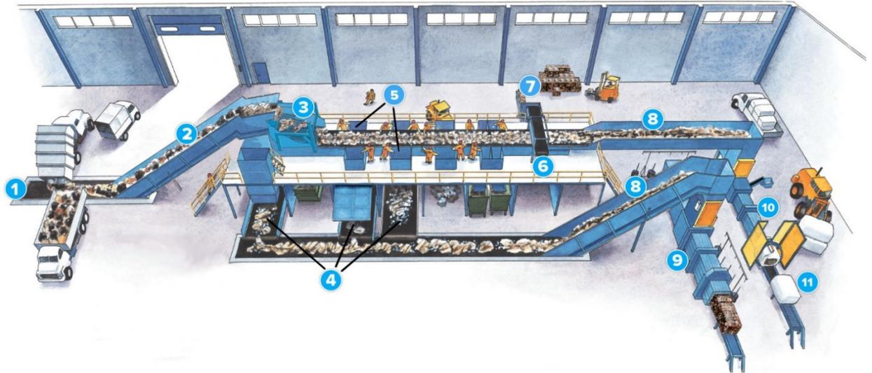
Figure 4. The example of human-operated waste segregation facility with separate conveyor line for paper waste.
