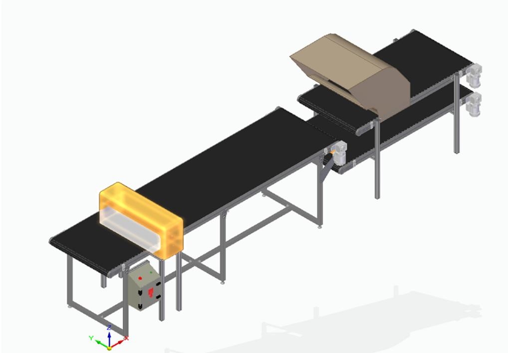
Figure 21. Conveyor line assembly. 3D model.
