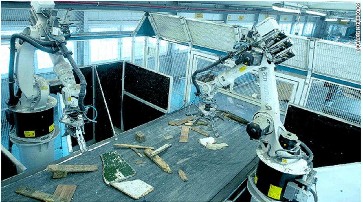
Figure 15. Alternative solution for manipulator segregation module on rotary axes
