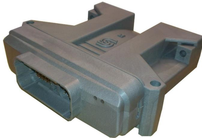
Figure 17. Danfoss Plus+1 50 pin controller [15].
