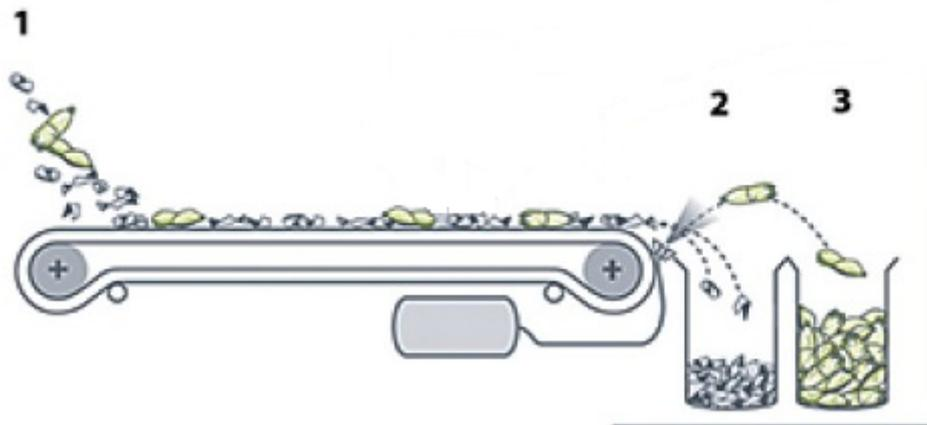
Figure 6. Schematic model of simple automated single line segregator.
