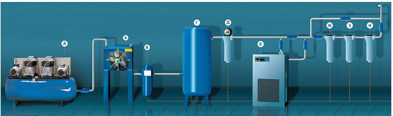
Figure 23. Pneumatic system air preparation module, in which (from left to right: Compressor; air cooler; cyclone type separator; reservoir; preliminary filter; air drier; intermediate with condensate remover; oil catching filter; coal filter) [13].
