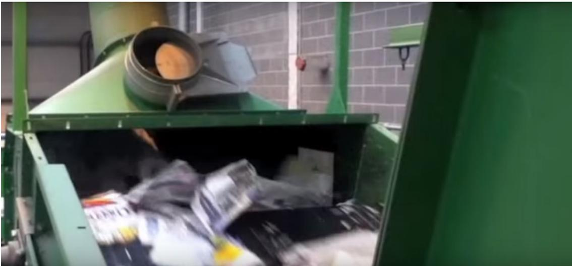
Figure 19. Paper separation with air jet
