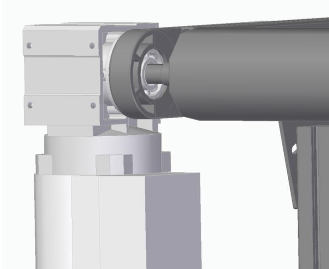
Figure 29. Tractive drum and motor reducer.
