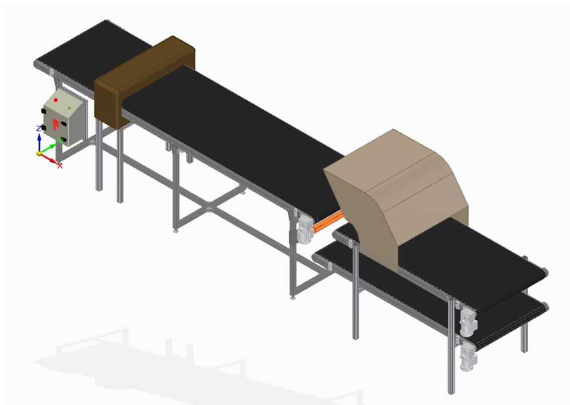
Figure 26. Conveyor line assembly. 3D model.
