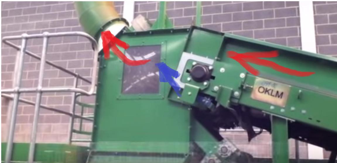
Figure 20. High-velocity air flow separation module. White paper moves shown with red. Air jets shown with blue.
