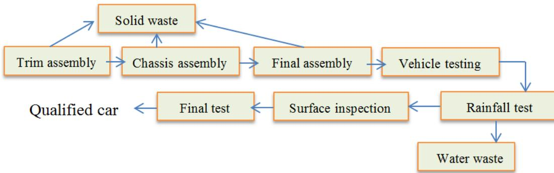
Figure 13, Process and problem of assembling [18] [26]
