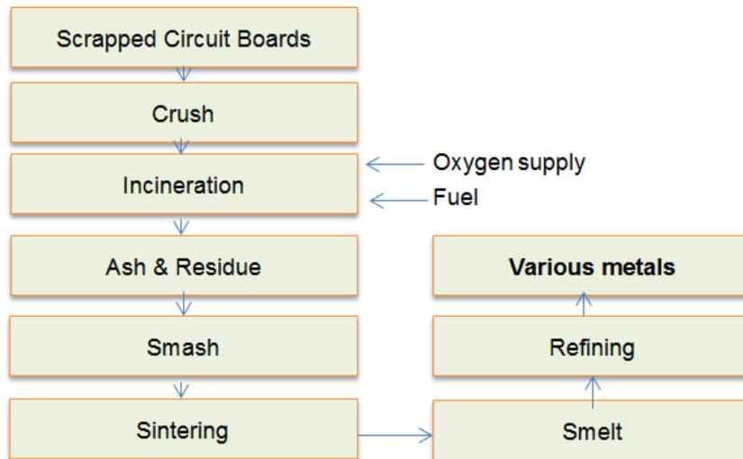
Figure 23, Incineration method of electronic remanufacturing
