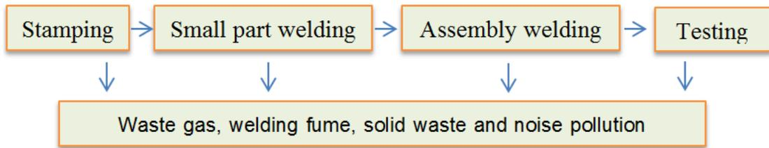
Figure 10, Process and problem of welding [18] [26]
