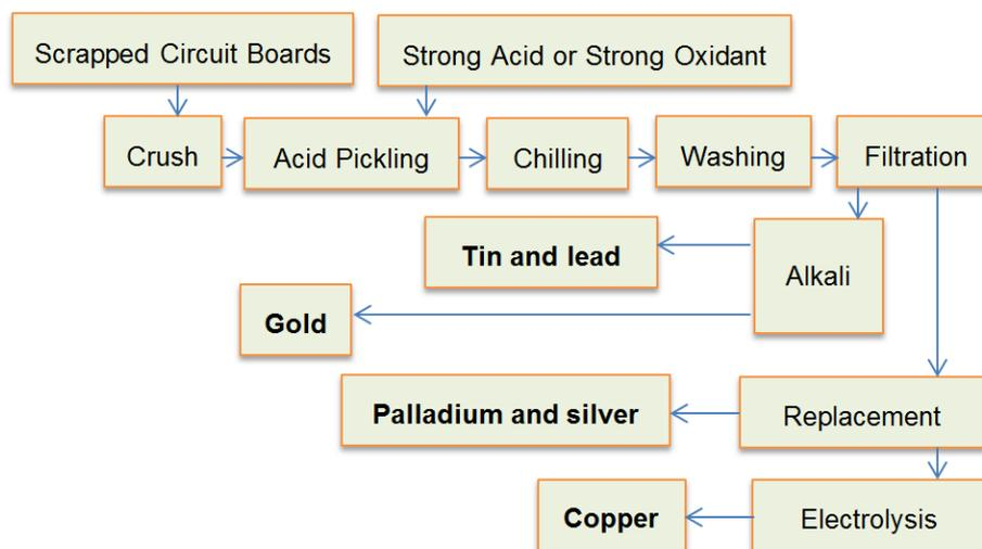
Figure 22, Chemical approach process of electronics remanufacturing
