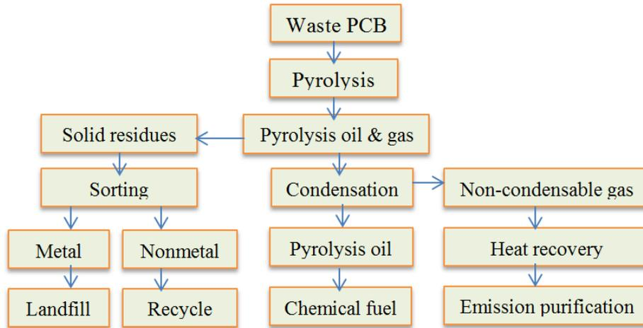
Figure 24, Pyrolysis method of electronic remanufacturing
