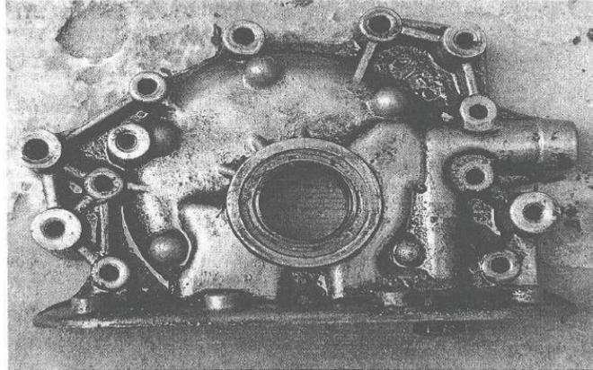
Figure 17, Engine cover after burning [27]
