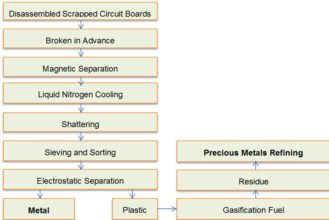
Figure 21, Process Routing of Physical Method
