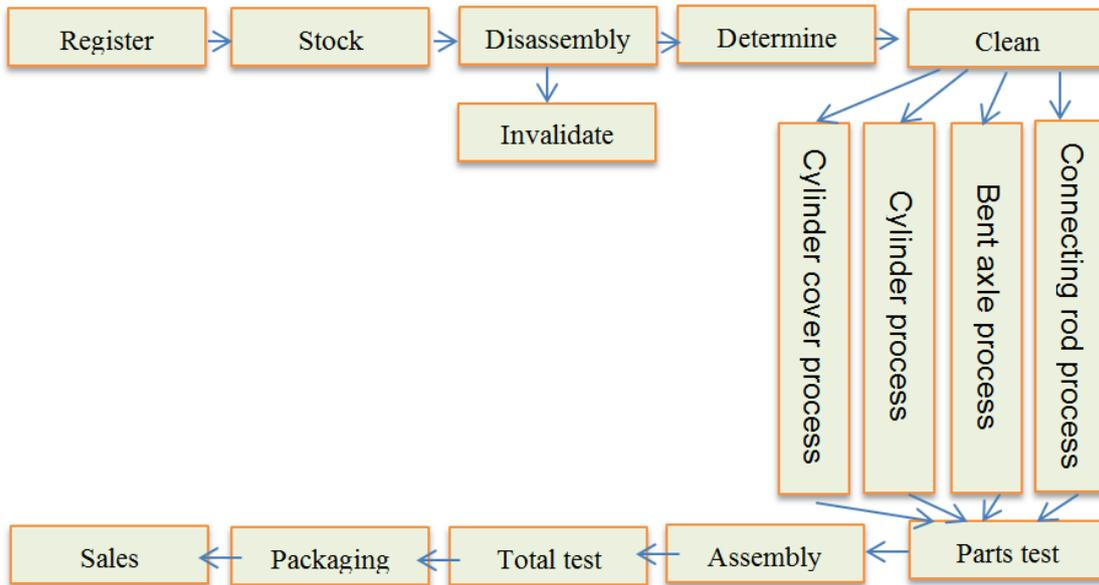
Figure 15, Process flow of engine remanufacturing [27]
