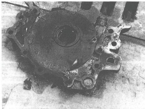
Figure 16, Engine cover before cleaning [27]
