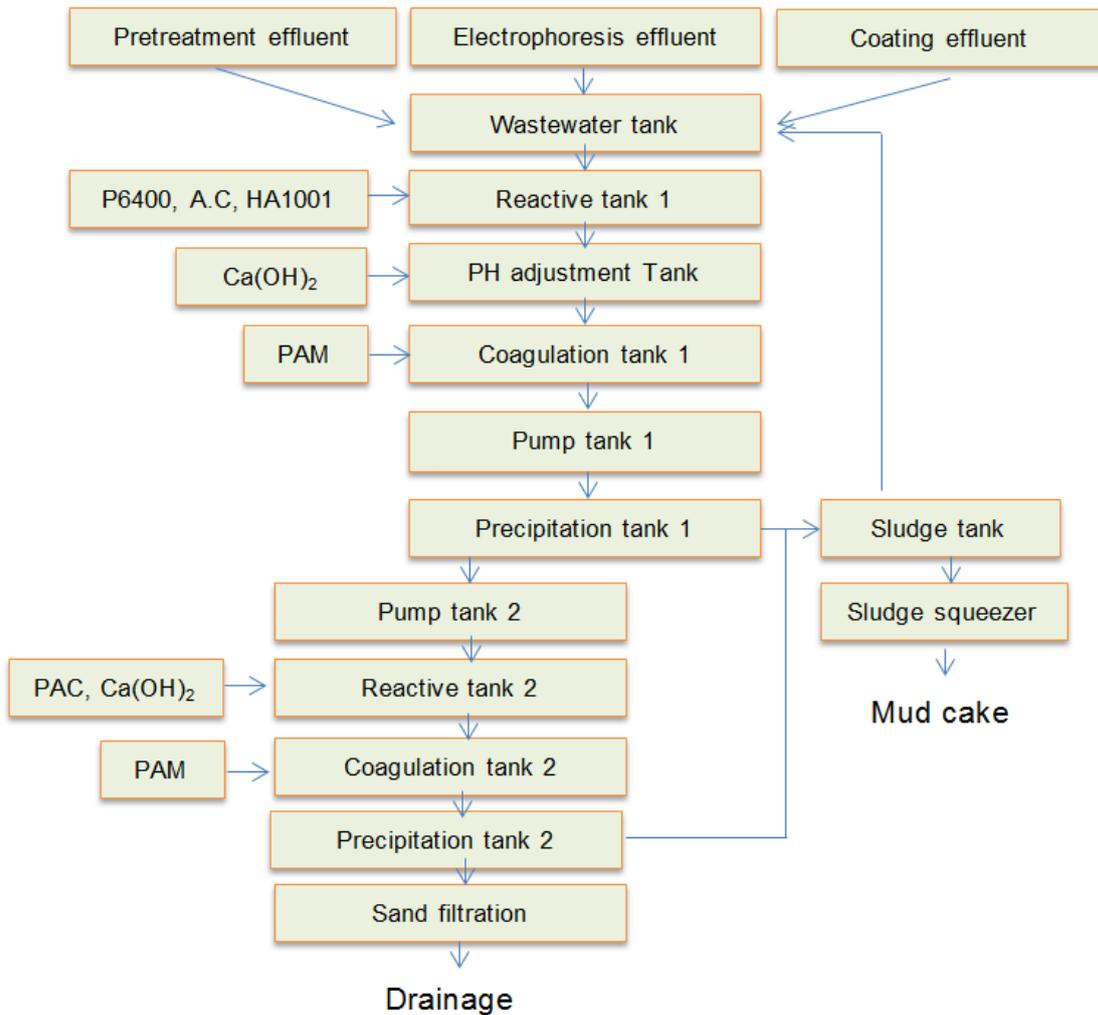
Figure 12, Green circulation processing flow of Coating Effluent [18] [26]
