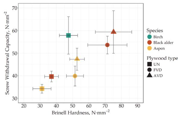
**Figure 7.** Plywood surface hardness vs. screw withdrawal capacity.
