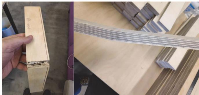
**Figure 4.** Test pieces after bending tests, showing brittle failure in black alder (left), and ductile failure in aspen (right) plywood.
