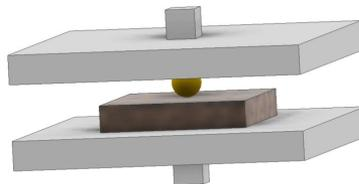
Figure 3. Brinell hardness test schema.
