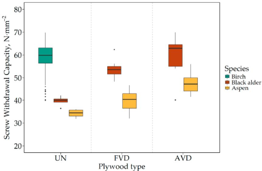
Figure 5. Average screw withdrawal capacity values for the tested plywood types.
