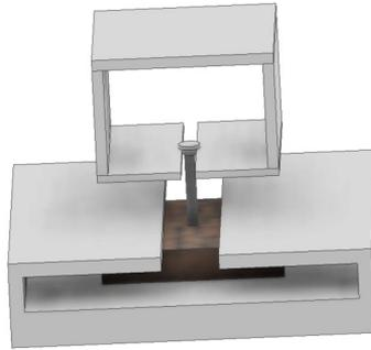
Figure 4. Screw withdrawal test schema.
