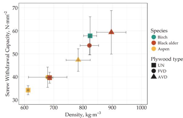
**Figure 6.** Plywood density vs. screw withdrawal capacity.
