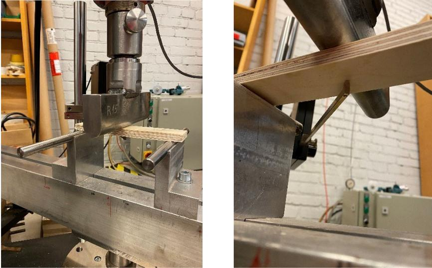
Figure 2 Bending strength (MOR) and modulus of elasticity (MOE) determinations.
