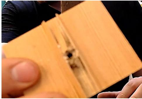
*Figure 6. Screw withdrawal test applied sample.*
