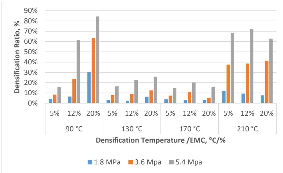
Figure 12. Densification ratio of samples in various pressing temperature, pressing pressure and initial EMC conditions.
