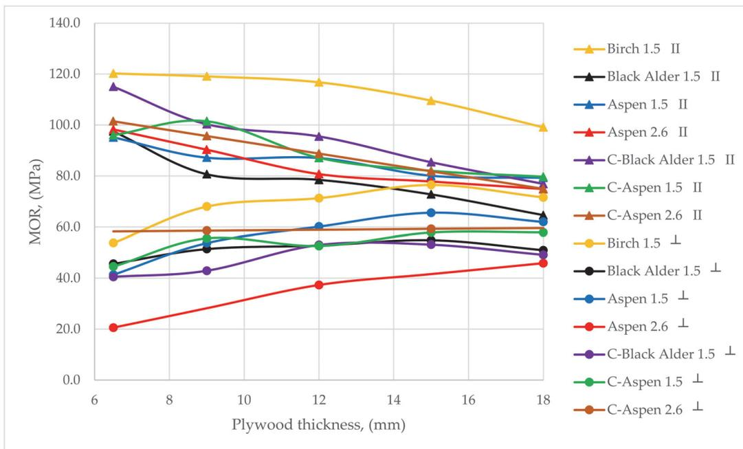
**Figure 3.** For different plywood types and thicknesses, MOR vs. thickness, in grain (II) and cross (⊥) direction. (Note: the same colour is used for both in grain and cross direction (lower values) for each plywood type).
