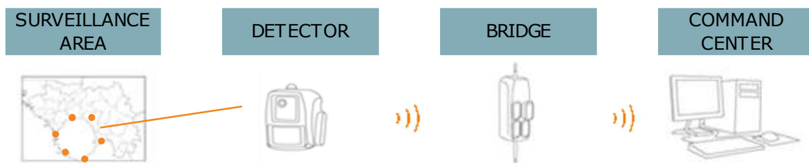
Figure 2.2 System Overview of the ReconEyez system [6]
