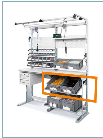
Figure 5.6 Exemplary Workstation with component storage marked in orange below the table [62]
