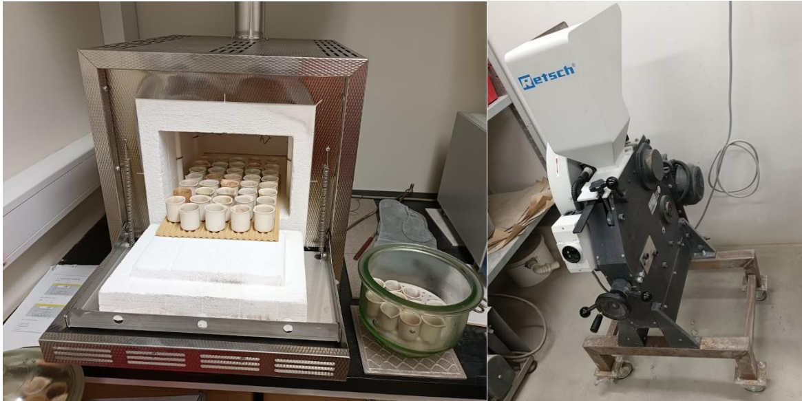
Figure 5. In the photo on the left samples are being placed in a blast furnace before heating the samples. In the photo on the right a Retsch jaw crusher is shown, which was used to crush the samples.
