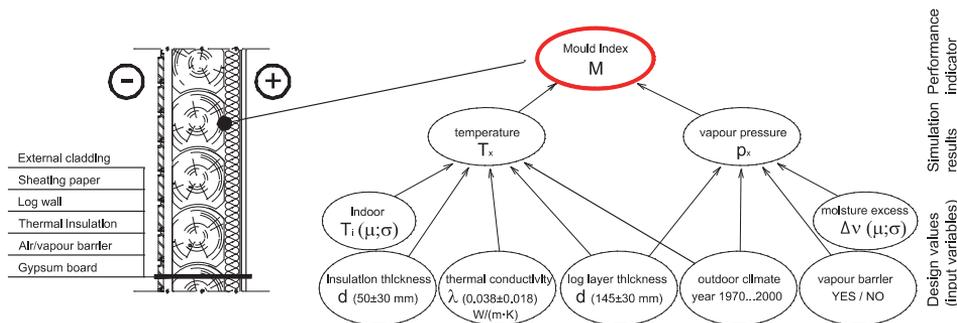
Figure 3.14 Design variables for the hygrothermal simulation model.
