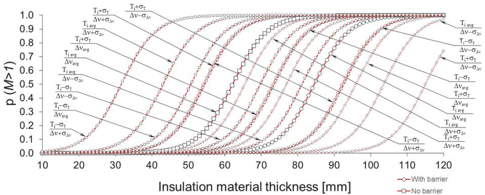
Figure 4.26 Change in the probability of mould index ( $M index > 1$ ) in the combination of different input variables with and without vapour barrier.
