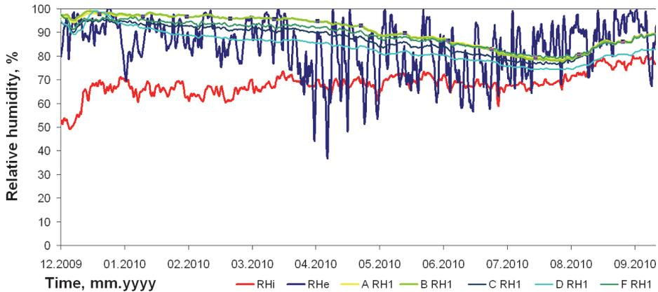
Figure 4.17 Measured RH inside the wall between the insulation materials.
