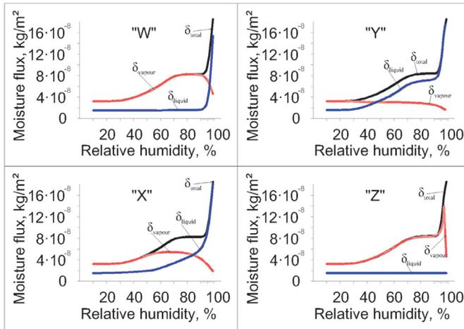
Figure 3.13 Total moisture flux in the middle of the material in different descriptions of water vapour  $\delta_{\text{vapour}}$  and liquid water  $\delta_{\text{liquid}}$ .
