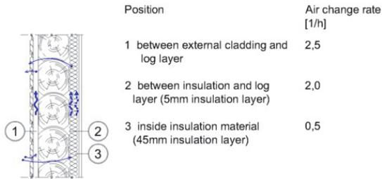
Fig. 3 Air change source in the material layers.
