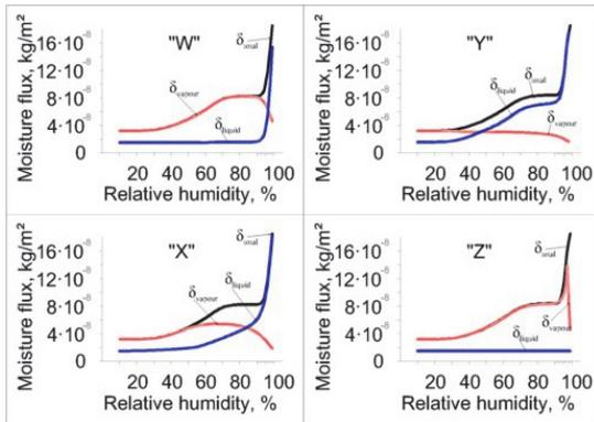
Fig. 2 Total moisture flux in the middle of the material in different cases of  $\mu$  and  $D_{ws}$ .
