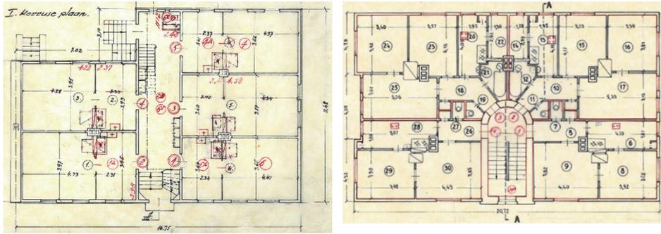
Figure 3.6 Floor plans of typical wooden apartment buildings (reference “A” and “B”).
