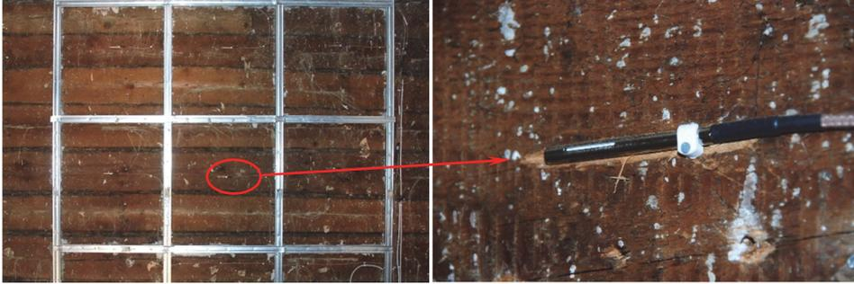
Figure 3.11 Temperature and relative humidity sensor on the log layer before the insulation material was added.
