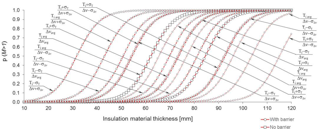
Figure 3. The change in probability of  $M\ index > 1$  in case of different input variables with and without vapour barrier.
