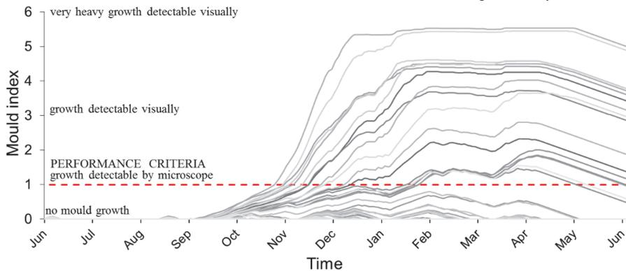
Figure 2. Calculated mould index between log and interior insulation layer of randomly generated 100 cases for one year period.
