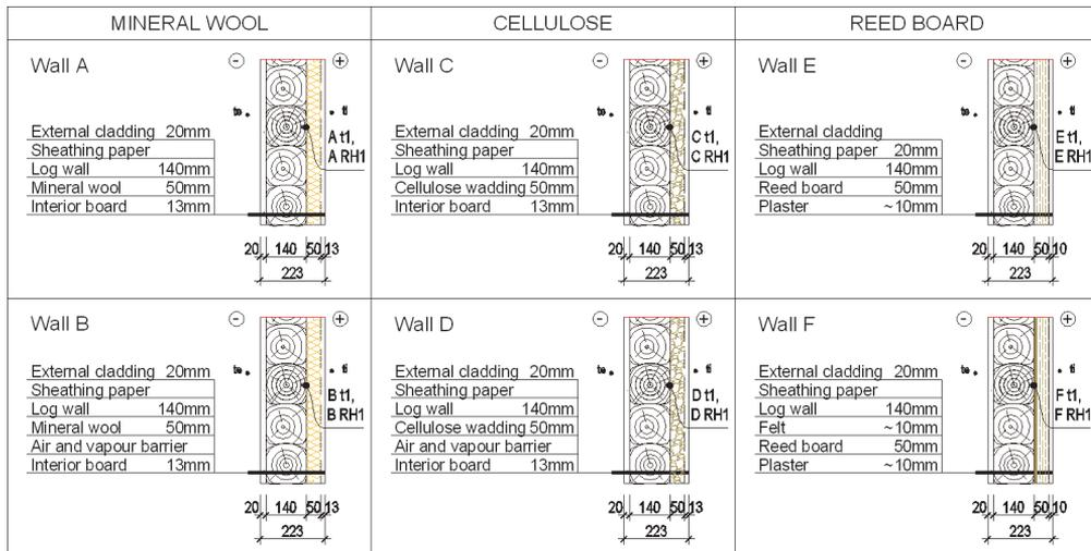
Figure 2. Sections of the studied test walls.
