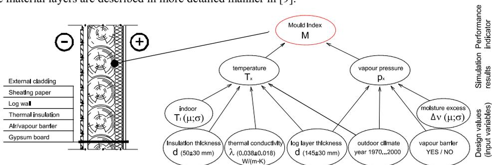
Figure 1. Design variables for the hygrothermal simulation model.
