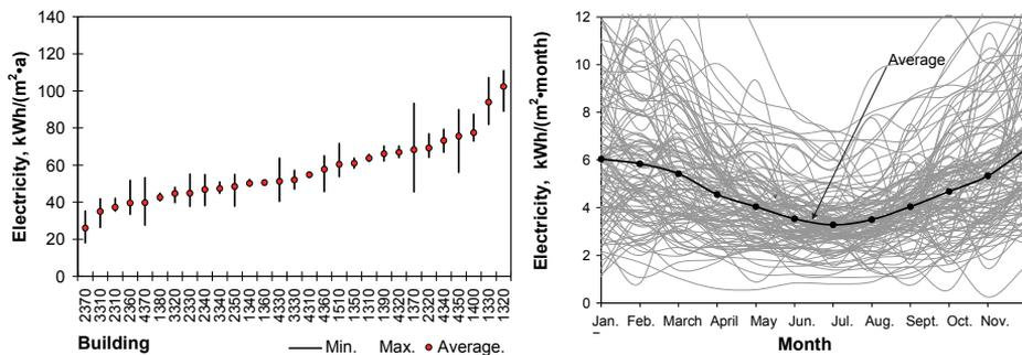
Figure 4.7 The average annual (left) and monthly (right) use of electricity in studied wooden apartment buildings.
