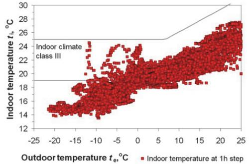
Fig. 5 The dependence of the indoor temperature on the outdoor temperature.
