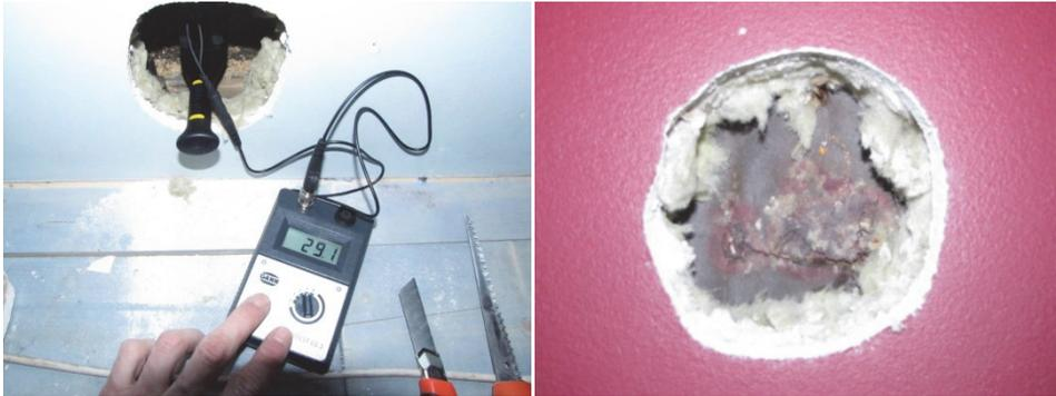
Figure 4.20 High moisture content of the log (left) and visual mould growth (right) in the case of log wall insulated from the interior side.
