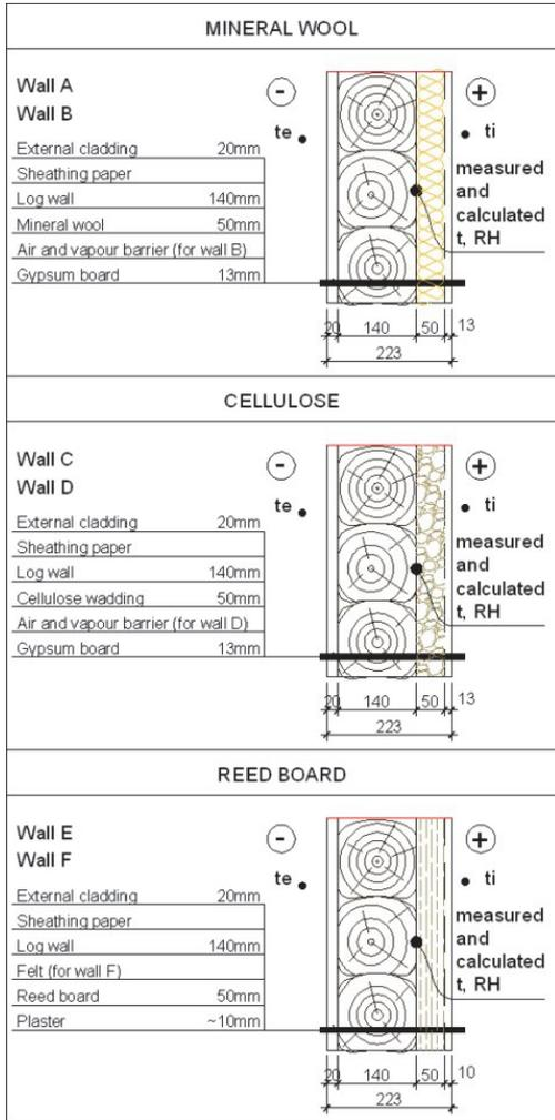
Fig. 1 The sections of the studied test wall.
