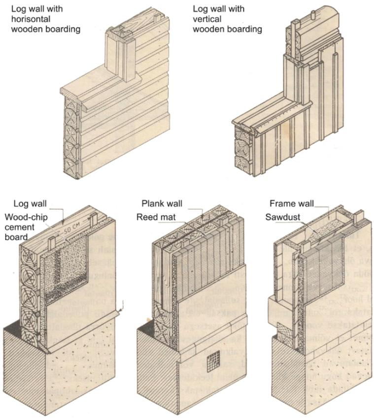
Figure 3.1 Typical external walls of wooden apartment buildings (based on Veski 1943).
