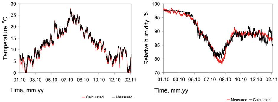
Figure 4.23 Calculated temperature and RH inside wall A between the insulation (mineral wool) and the log layer.
