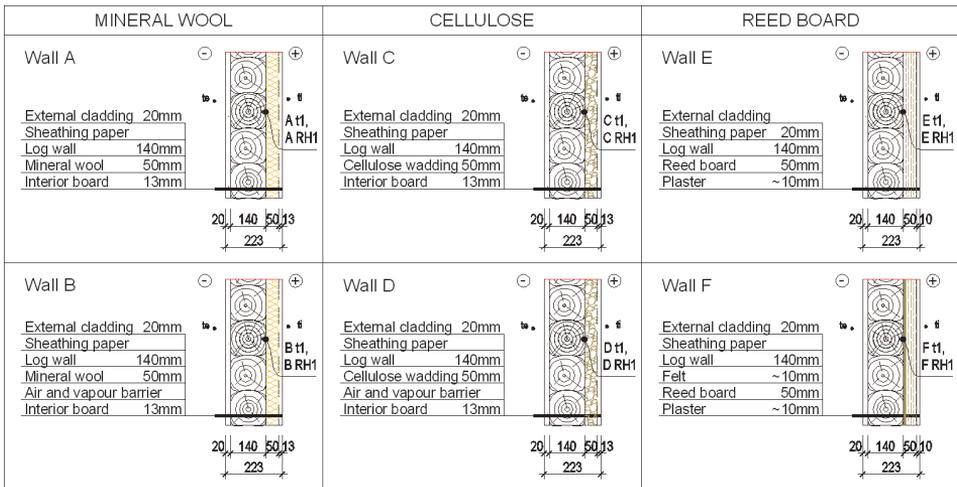
Figure 3.10 Sections of the studied test walls.
