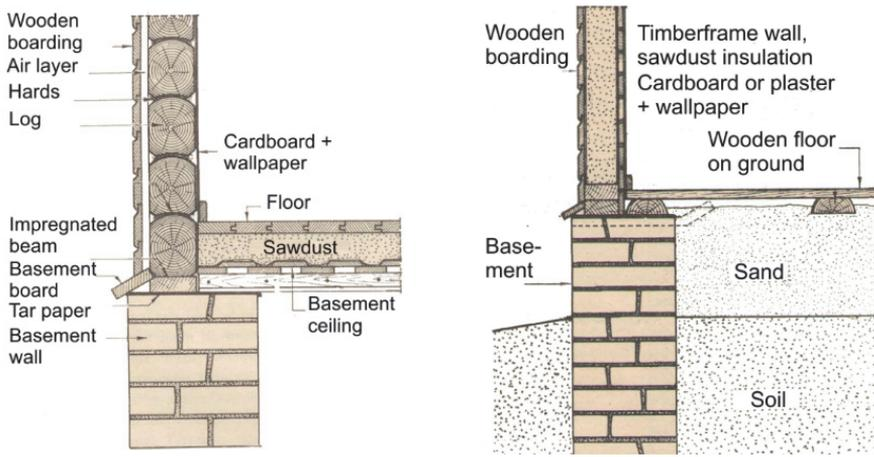
Figure 3.2 Connection of the external wall, basement and floor (building with a cellar (left); wooden slab on the ground (right)) (according to Veski (1943)).
