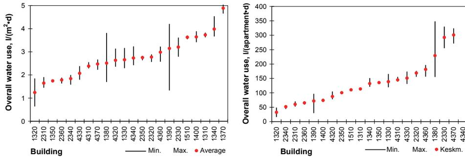
Figure 4.8 The daily average overall (hot and cold) water use in wooden apartment buildings.
