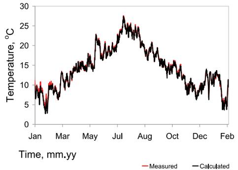
Fig. 13. Calculated temperature inside the wall E between the insulation (reed insulation mat) and log layer.
