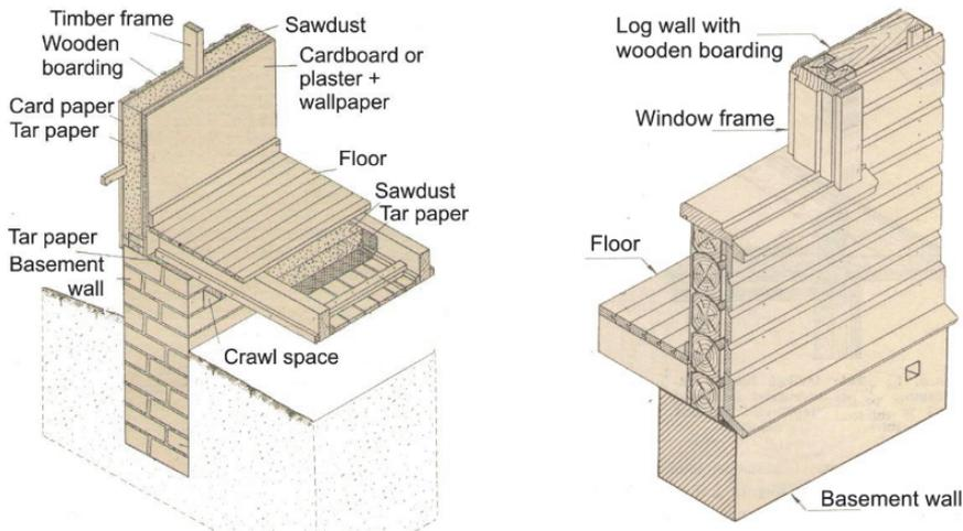
Figure 3.3 Connections of the exterior wall with floor (left) and window (right) (based on Veski 1943).
