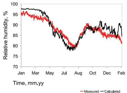
Fig. 14. Calculated relative humidity inside the wall between the insulation (reed insulation mat) and log layer.
