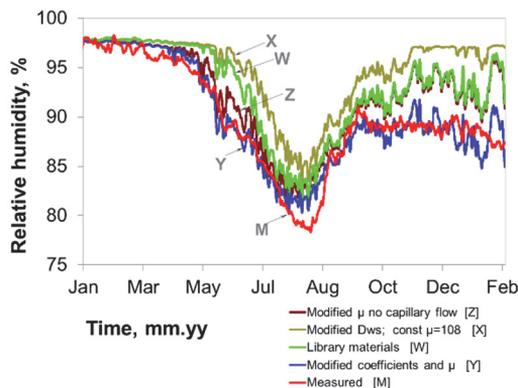
Figure 4.22 Calculated RH inside the wall A between the insulation (mineral wool) and the log layer with the air change rates.
