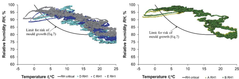
Figure 4.19 Temperature and RH conditions are favourable for mould growth for “green” insulations (left) and for mineral wool (right).
