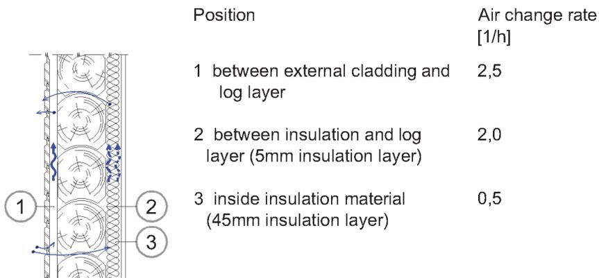
Figure 3.12 Air change source between the material layers.
