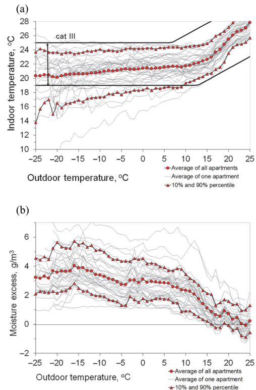
**Fig. 2.** Dependence of indoor temperature (a) and moisture excess (b) measurement results on the outdoor temperature (Sanders, 1996).
