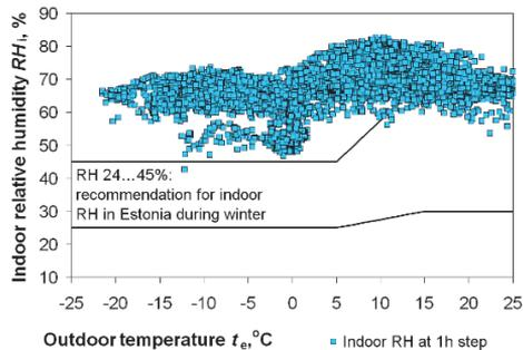
Figure 4.15 Dependence of the indoor RH on the outdoor temperature. Reference point to assess the hygrothermal performance of the internally insulated wall was between the original log and the internal insulation, see Figure 3.11 left.
