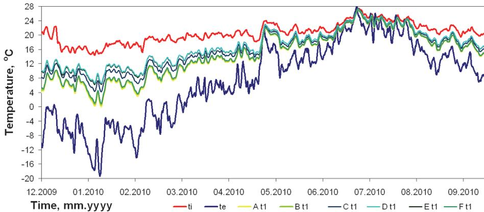
Figure 4.16 Measured temperatures inside the wall between the insulation materials.
