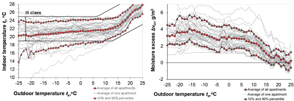
Figure 4.1 The dependency of indoor temperature (left) and moisture excess (right) measurement results on the outdoor temperature.
