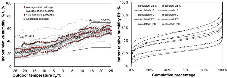
Figure 4.3 Indoor air RH measurement results (left) and comparison of measured and calculated RH (right) at different outdoor temperatures.
