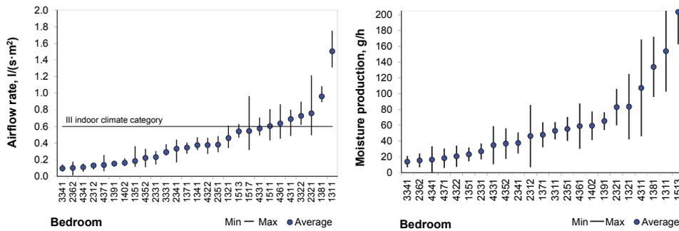
Figure 4.4 Airflow rate (left) and moisture production (right) in bedrooms during winter period.
