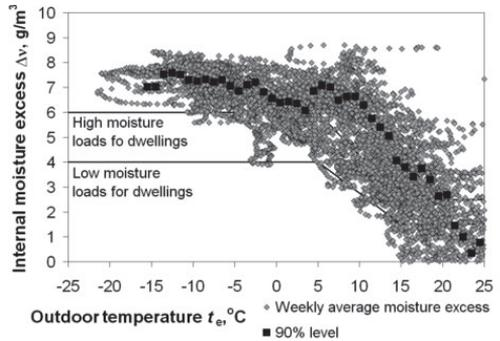
Fig. 6 The dependence of the moisture excess on the outdoor temperature.
