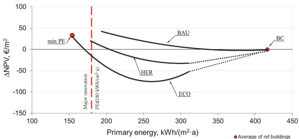
Figure 4.13 Comparison of renovation packages considering different attitudes and requirements.
