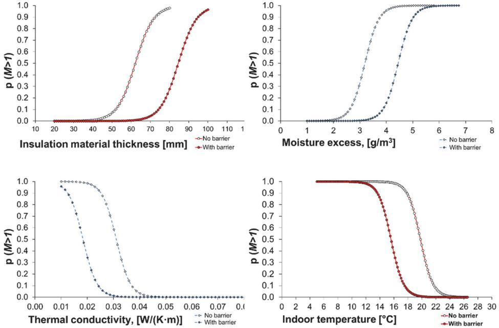
Figure 4.25 The change in probability of mould index ( $M index > 1$ ) for different variables with and without vapour barrier.
