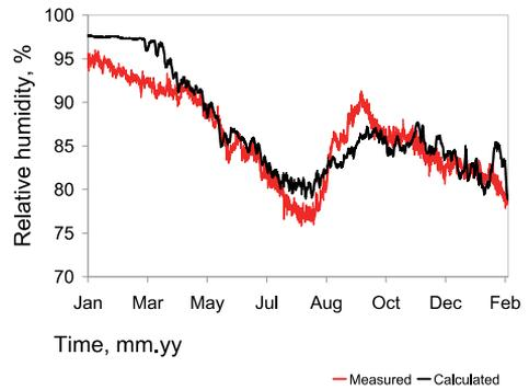
Fig. 12 Calculated relative humidity inside the wall C between the insulation (cellulose wadding) and log layer.
