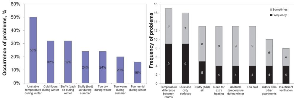
Figure 4.6 Occurrence (left) and frequency (right) of the problems based on the questionnaire.
