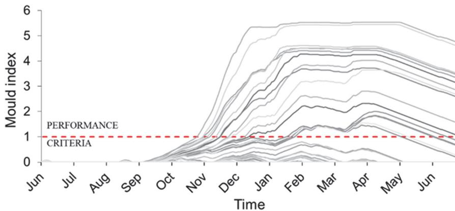
Figure 4.24 Calculated mould index between the log and the interior insulation layer of randomly generated 100 cases for a one-year period.
