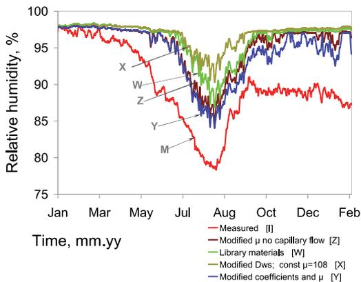
Fig. 7 Calculated relative humidity inside the wall A between the insulation (mineral wool) and log layer.
