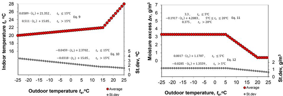
Figure 4.2 Indoor temperature (left) and moisture load design curves for historic wooden apartment buildings.
