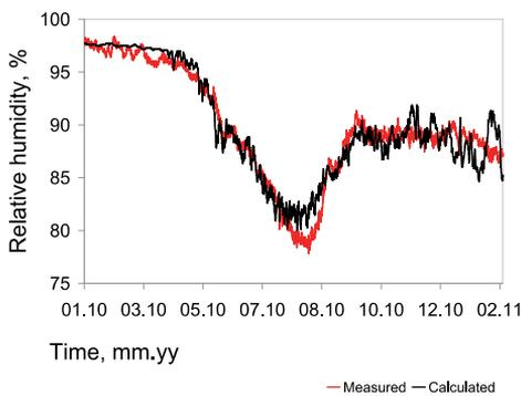
Fig. 10 Calculated relative humidity inside the wall A between the insulation (mineral wool) and log layer with changed transport coefficients.
