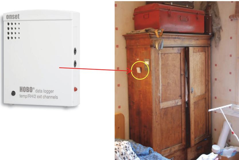
Figure 3.7 Measurement of indoor temperature and RH in a bedroom: used logger (left) and location in bedroom (right).
