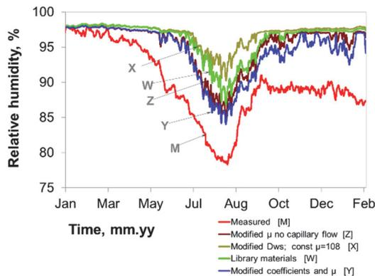
Figure 4.21 Calculated RH inside the reference wall “A” between the insulation (mineral wool) and the log layer.
