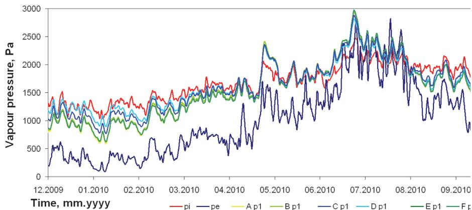
Figure 4.18 Measured water vapour pressure inside the wall between the insulation materials.
