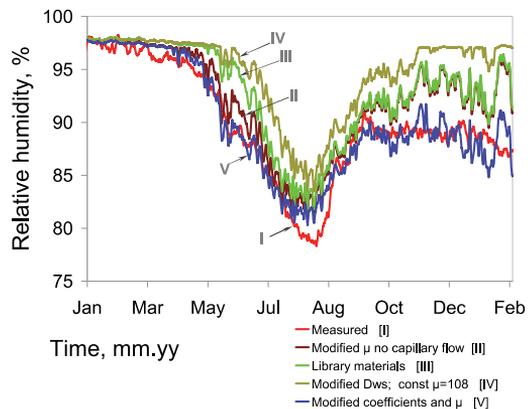
Fig. 8 Calculated relative humidity inside the wall A between the insulation (mineral wool) and log layer with the air change rates.
