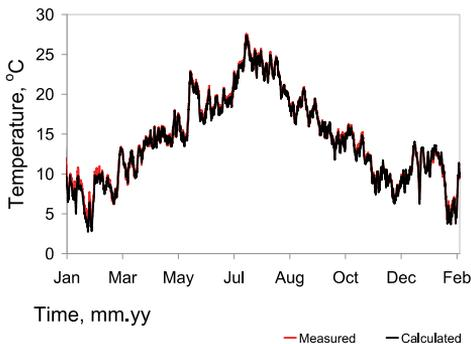
Fig. 11. Calculated temperature inside the wall C between the insulation (cellulose wadding) and log layer.
