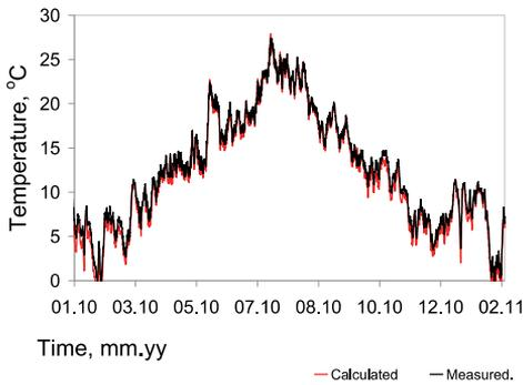
Fig. 9 Calculated temperature inside the wall A between the insulation (mineral wool) and log layer.
