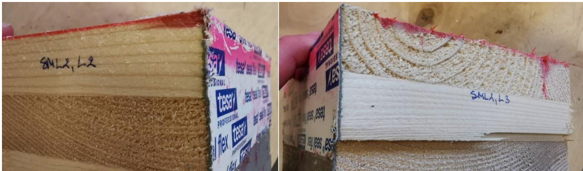
Figure 3.10 Sample with mastics and tape covered edges and incisions. Some of the water has gotten through the tape in the left, and in the right, tape and mastics have done a great job of keeping the water away from the wood.
