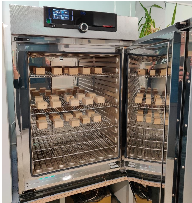
Figure 2.9 Test pieces placed in an oven
