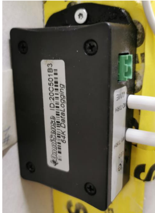
Figure 2.2 Transmitter used in Omnisense system
