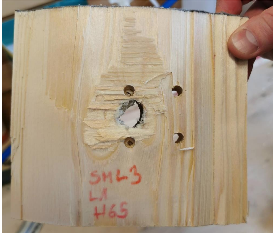
Figure 3.12 Oven-dry test piece with the knot placed between two electrodes
