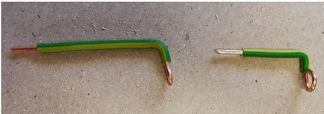
Figure 2.3 Insulated copper wire electrodes
