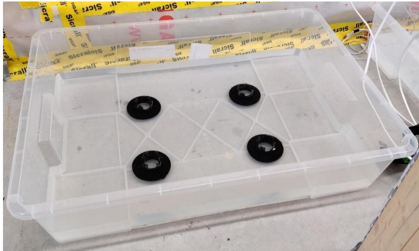
Figure 2.7 Plastic container with dashboard supports on the bottom
