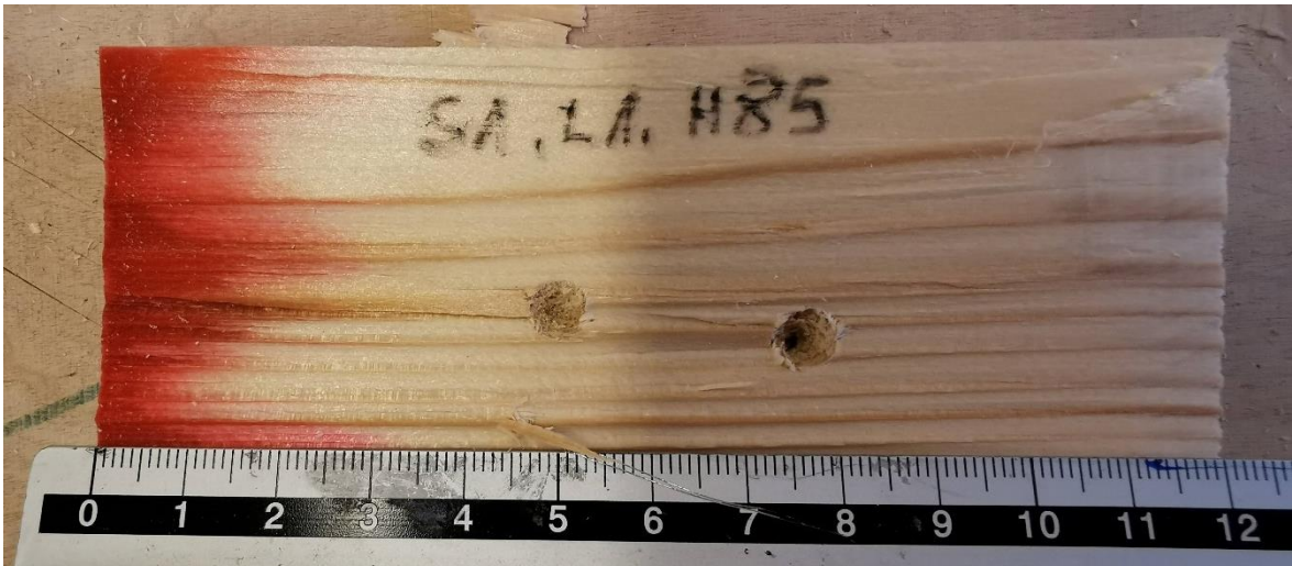
Figure 3.7 Oven-dry method sample piece shows how far the water has gotten into the first layer.
