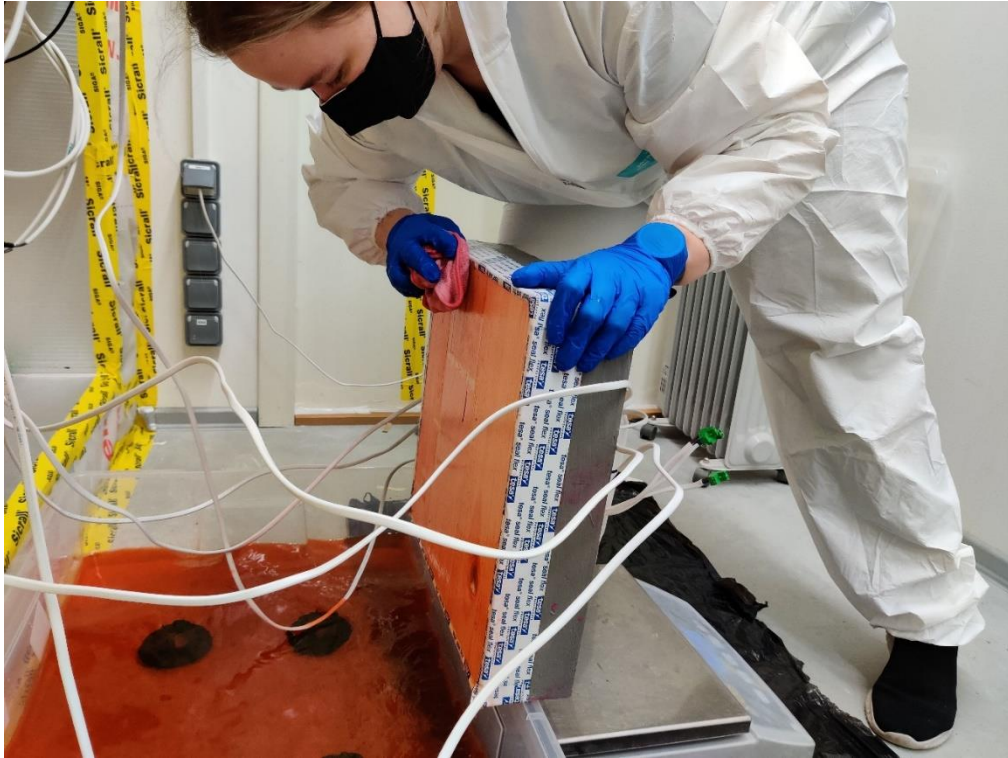
Figure 2.10 Blotting of the excess water of the sample before weighing
