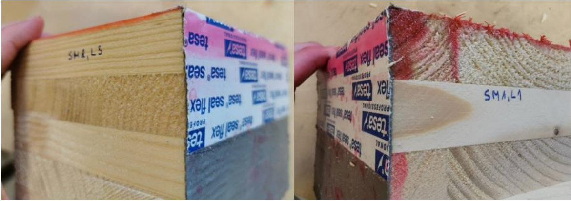
Figure 3.8 Pieces cut from a sample with mastic and tape covered edges. The left one shows the first layer in the longitudinal direction, with no water leakage from the edge and the right one in the radial direction, where some water has gotten through the tape and mastic and between two pieces of wood.
