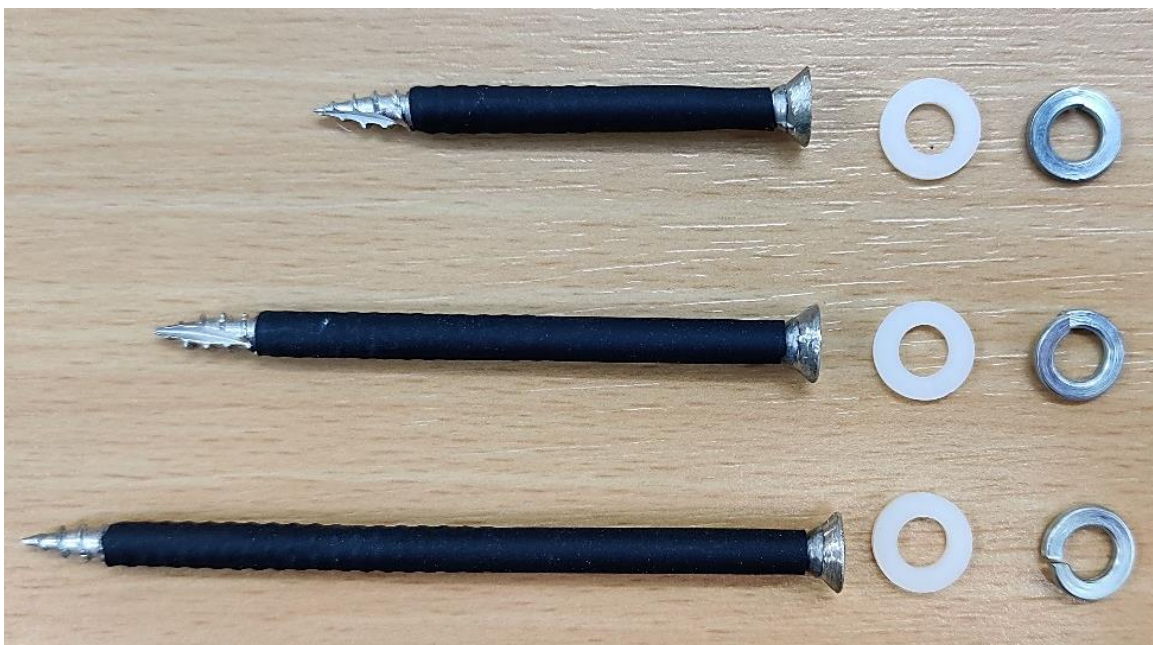
Figure 2.4 Insulated screw electrodes with plastic and spring washers
