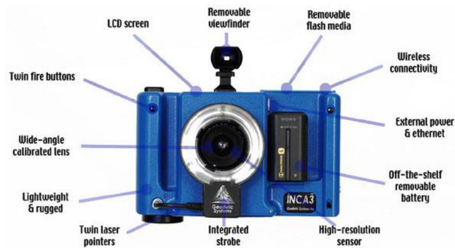
Figure 2.2. “INCA 3a+” camera for industrial photogrammetry
