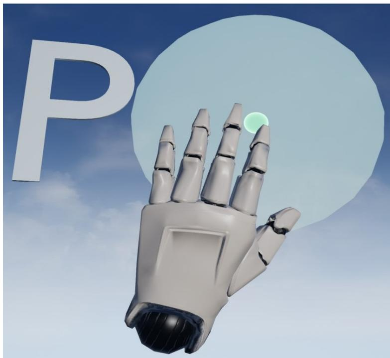
(b) CollisionSphere on controller overlaps the Control Sphere, controller model changes to “palm” and the sphere can be grabbed.
