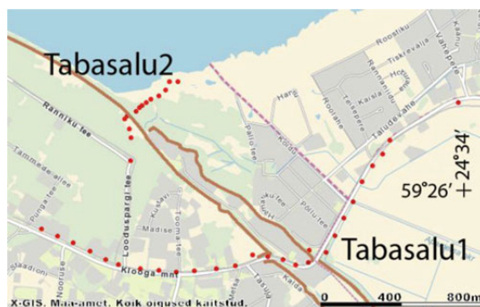
Fig. 1 Detailed gravity measurement profiles Tabasalu1 and Tabasalu2 (depicted by red dots) crossing the North-Estonian Klint (depicted by the brown line) near seashore (Color figure online)
