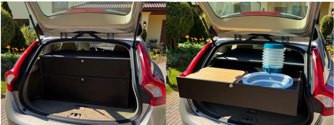
Figure 6.2. Completed prototype. On the left, the drawer system is closed. On the right, additional features. [Author's collection]
