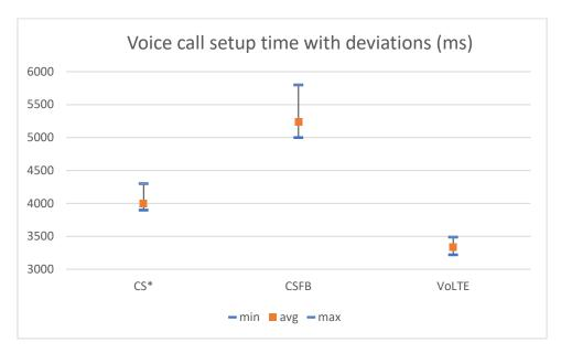
Figure 24. Voice call setup delay times. CS\* is estimated value.
