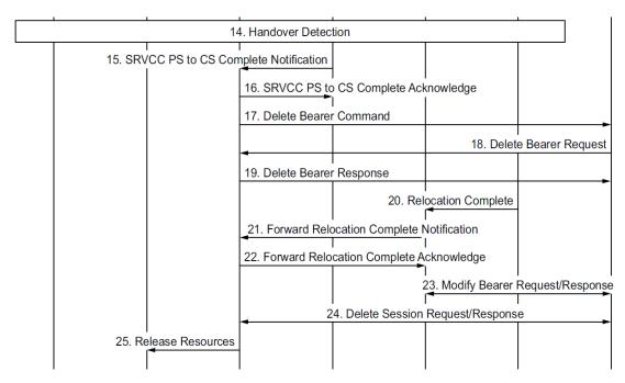
Figure 20. SRVCC Handover completion. [7]
