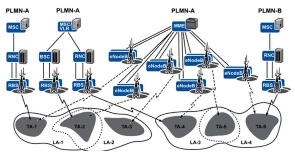
Figure 13. TA-LA mapping example [7]
