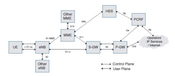
Figure 3. EPC detailed level architecture [7]
