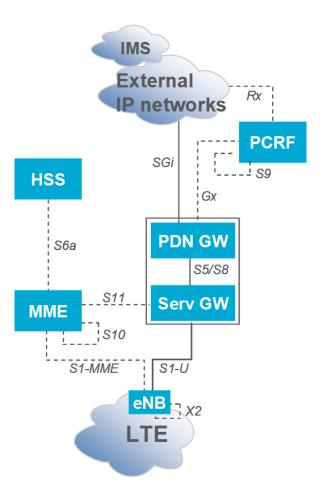
Figure 5. EPC main control plane and user plane interfaces. [7]
