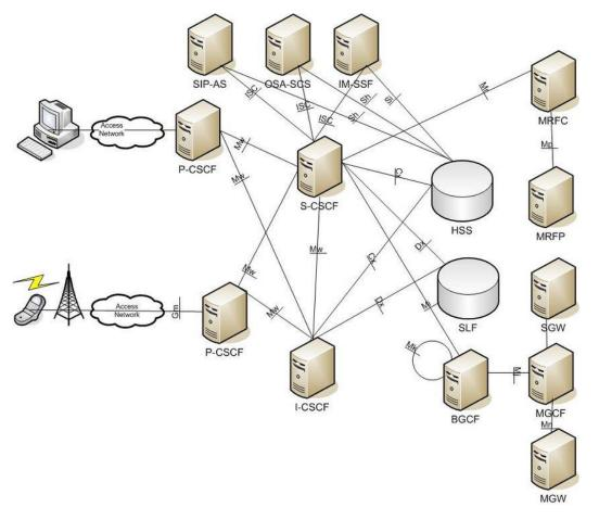
Figure 10. IMS core detailed architecture[14]
