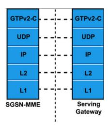
Figure 6. S11 interface protocol stack. [7]
