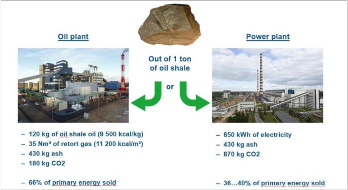
Figure 13. Different ways of oil shale use [19]
