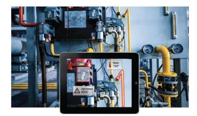
Figure 2.6. Augmented Reality maintenance screen. The digital data is aligned with the real world elements  $[\underline{13}]$ .
