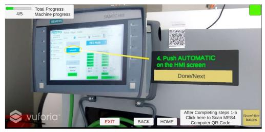
Figure 3.18. AR application ASRS step 4/5
