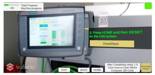
Figure 3.17. AR application ASRS step 3/5
