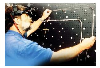
Figure 2.5. Researchers at Boing looking through HMD guiding the assembly of wire bundles [12]
