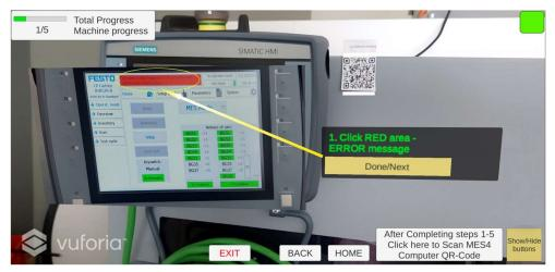
Figure 3.15. AR application ASRS step 1/5
