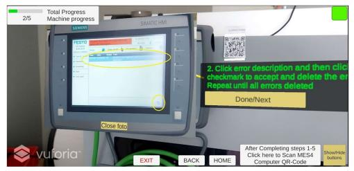
Figure 3.16. AR application ASRS step 2/5
