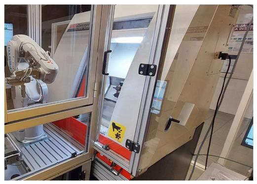
Figure 2.13. Turning machine EMCO Concept Turn105
